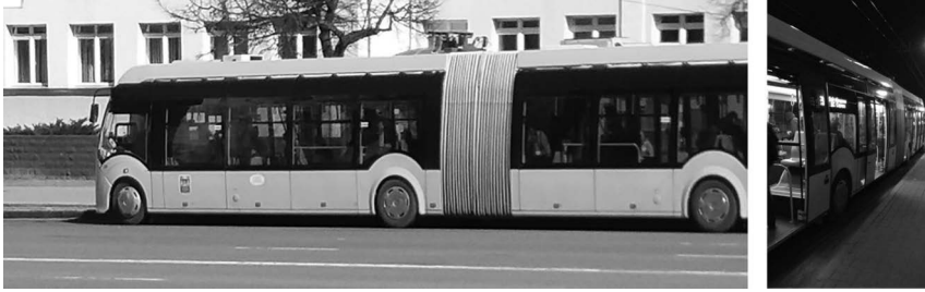
FIGURE 5.1 A commercial supercapacitor-powered electric bus in operation. The bus's supercapacitor requires approximately 5 minutes of charging, providing 12–17 km of driving distance. The main advantage of such a system is a potentially “unlimited” number of charging-discharging cycles within the relevant vehicle lifetime.
