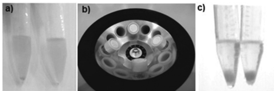
FIGURE 5.12 Photographs of the sequence of the separation of the nanoparticle solution in two tubes (a) to centrifuge (b) and decant (c).
