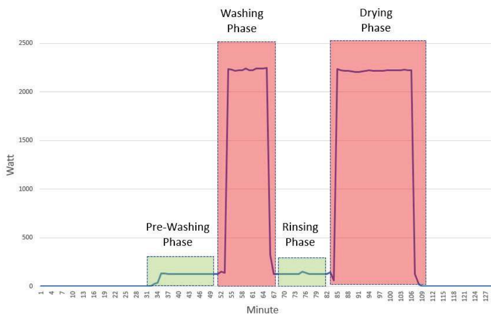
Figure 9. Example of power consumption of a dishwasher.
