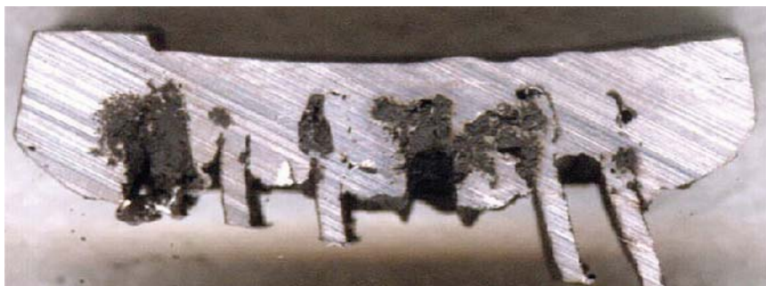
Figure 12.26 Section through the positive group bar of a starter battery after a standard corrosion test. For some electrodes the contact to the group bar is completely intact, for others a corrosion attack along the terminal lugs and further corrosive destruction of the group bar can be seen. Source: Courtesy of E. Cattaneo.
