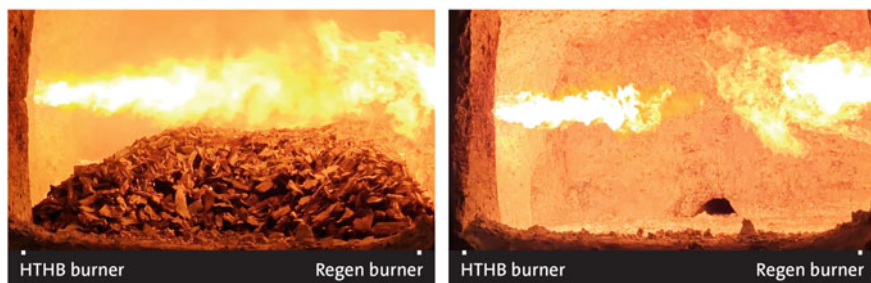
Fig. 5 Flame images from reverb furnace: a start of the cycle, b end of the melt cycle
