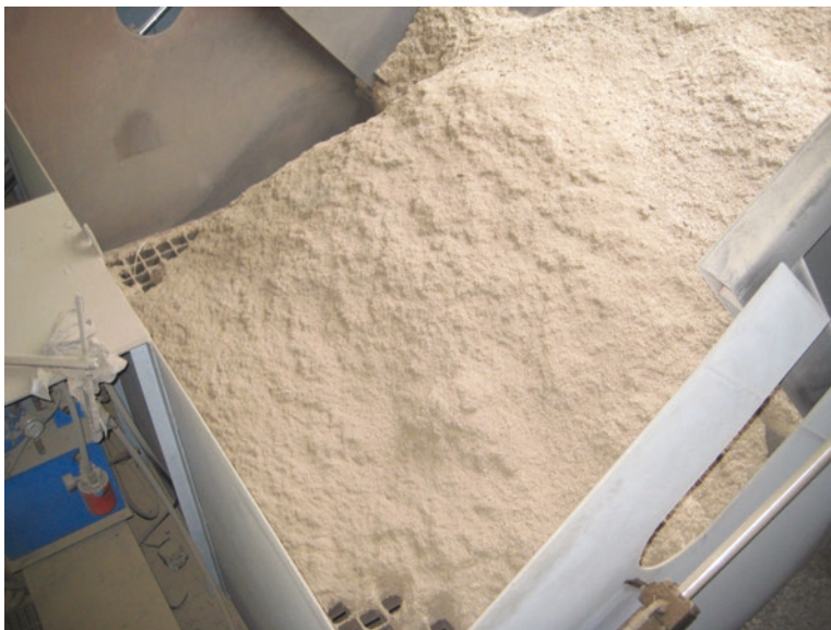
Fig. 13.2 Ground switch grass loaded into a fuel bunker. (Photo by EV Johnstonbaugh)
