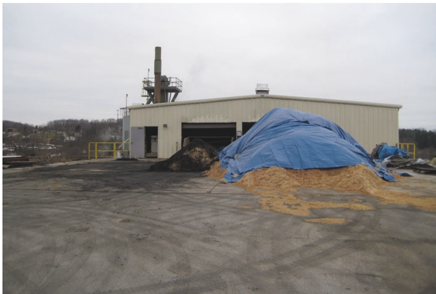
Fig. 13.5 Ground switch grass awaits co-firing with waste coal at a fluidized bed combustion plant. (Photo by EV Johnstonbaugh)
