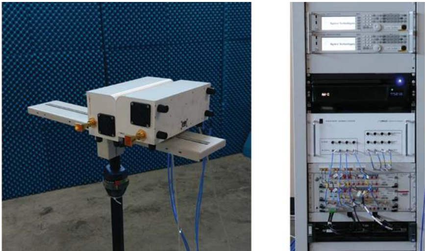
Figure 17.3 The CREW equipment. The radar RF module comprising a single transmitter and receiver is shown on the left-hand side. The waveform generators, digitizers, based band converter and local oscillator are mounted in a standard rack, shown on the right-hand side. Figure taken from [13]. ©2016 IEEE.
