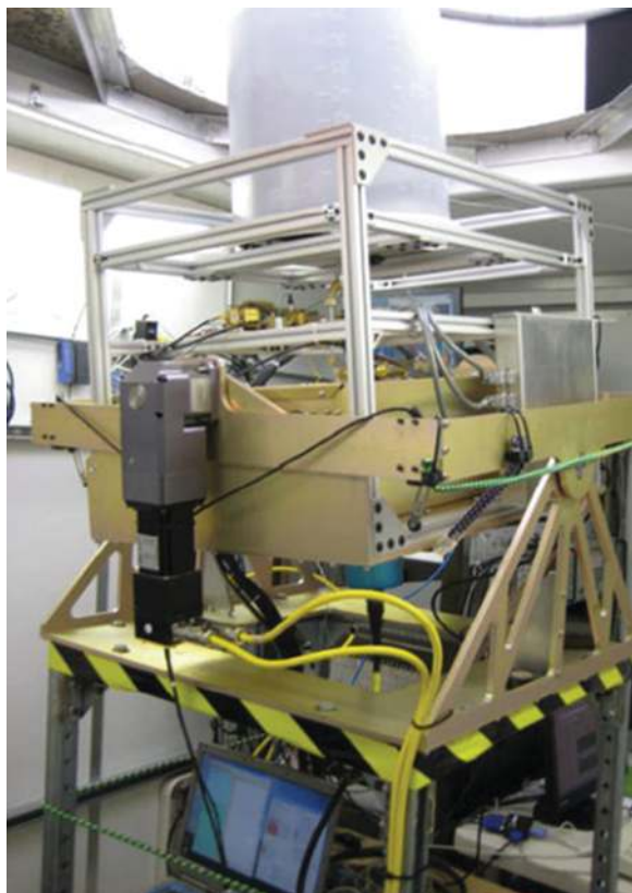
Figure 8.22 An example of a stabilized platform with a radar and sitting below a hatch (from [144]). Other solutions are given in [121,141,145]. Used with permission.
