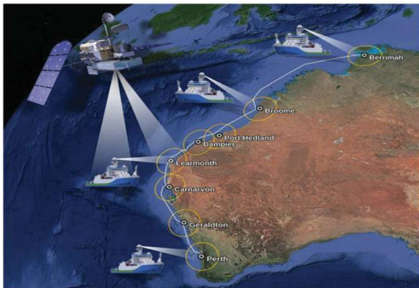
Figure 8.11 The concept of shipborne (OceanPOL on the R/V Investigator) and ground-based inter-comparisons for calibration using the GPM Ku-band spaceborne radar. The 150 km radius is shown by a yellow circle and the ship track by a white line. © 2021 Google Earth Map Data: SIO, NOAA, US Navy, NGA, GEBCO; Map image Landsat/Copernicus (after [68]).
