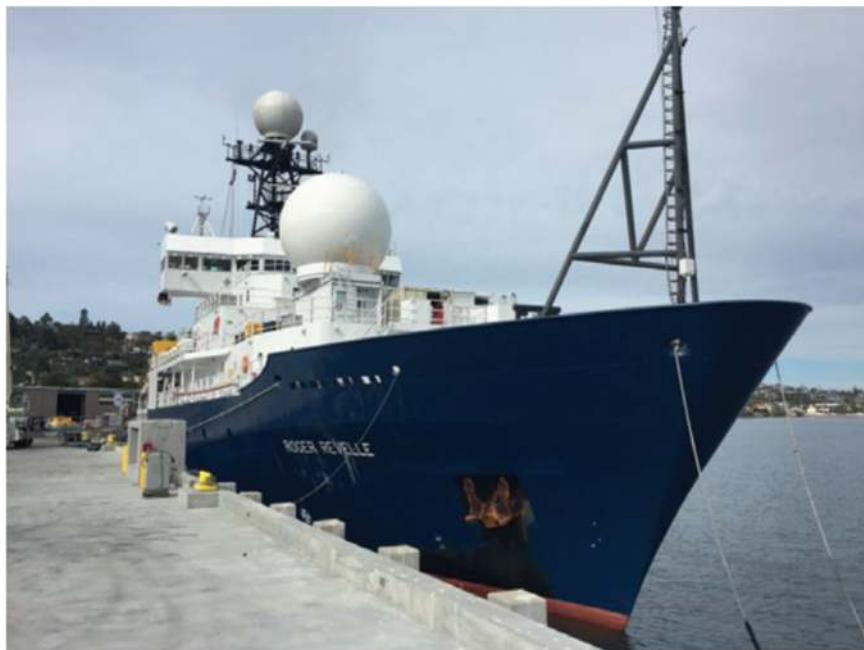
Figure 8.8 Photo of SEA-POL mounted on the foredeck of the R/V Roger Revelle in San Diego before departing on the SPURS-2 cruise. SEA-POL is the large radome near the bow of the ship. The smaller radome mounted above the bridge houses the ship's satellite communications antenna. [Credit: Steven Rutledge; this figure is reprinted from [66] under the terms of the Creative Commons Attribution 4.0 International License ( https://creativecommons.org/licenses/by/4.0/ ).
