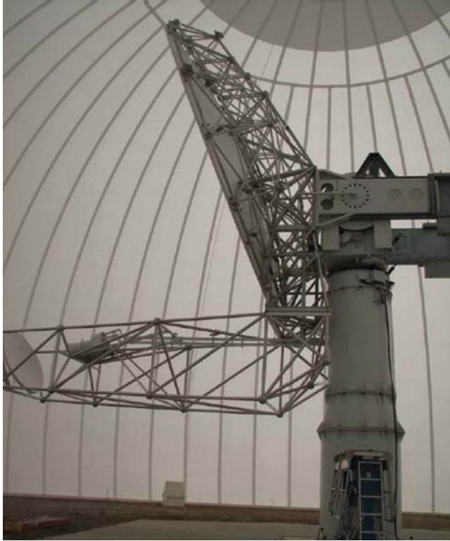
Figure 1.1 The Colorado State University-Illinois State Water Survey (CSU-CHILL) S-band weather radar with a 9-m Gregorian design antenna shown here with the pedestal and radome. Photo credit: Kumar Vijay Mishra, with permission from CSU-CHILL Co-Principal Investigator V. N. Bringi.
