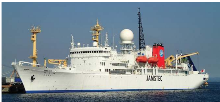
Figure 8.9 Photo of R/V Mirai with the upgraded M-POL radar mounted at the middle of the vessel
