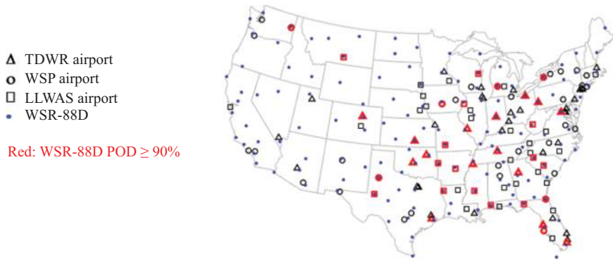
Figure 10.11 US airports with wind shear detection systems and WSR-88D locations. Red outlines on wind shear detection system icons indicate that WSR-88D siting supports microburst probability of detection equal to or greater than 0.9. The following TDWR airports are also equipped with LLWAS: Atlanta (ATL), Denver (DEN), Dallas/Fort Worth (DFW), New York-LaGuardia (LGA), Orlando (MCO), New Orleans (MSY), Chicago-O'Hare (ORD), St. Louis (STL), and Tampa (TPA).
