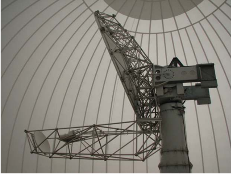
Figure 2.2 CSU-CHILL radar Gregorian antenna.
