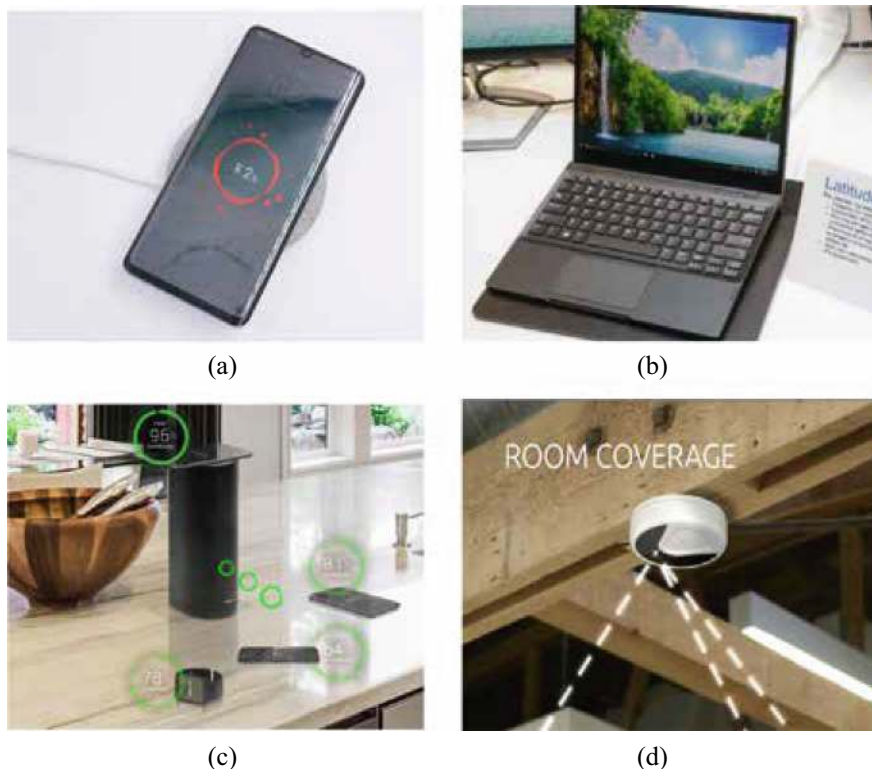
Fig. 1.10 WPT applications for portable electronic devices. a Huawei 27 W wireless fast charging. b Dell laptop wireless charging. c Wattup RF wireless charging. d Wi-charge infrared wireless charging
