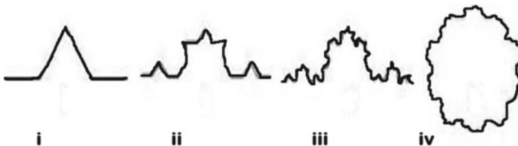
Fig. 9.1 Design steps involved in the patch design
