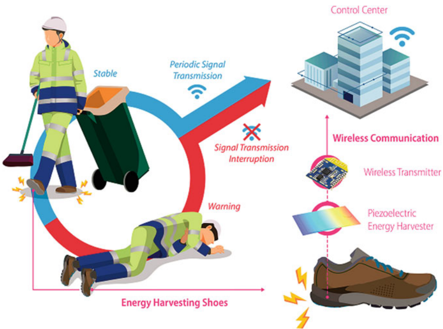
Fig. 1.6 Smart shoe based on PEH (Jeong et al. 2022)
