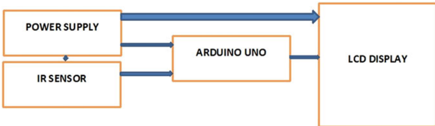
Fig. 7.4 Block diagram showing parking monitoring and sensing
