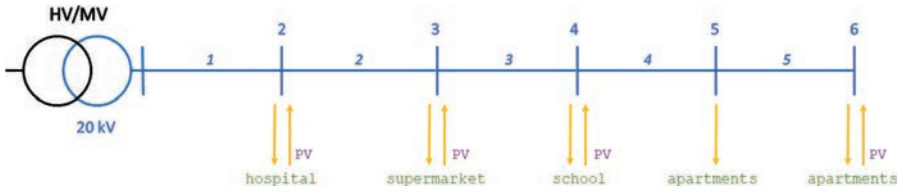
Figure 9.7 Simple MV network used for the tests
