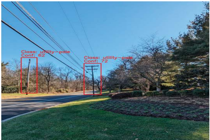
Figure 5.13 Typical scene of a roadway with bounding boxes around instances of utility poles.
