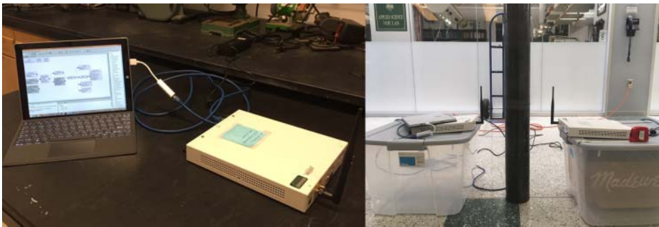
Figure 1.16 The portable, inexpensive, high-performance USRP is a scalable software defined radio platform that features a customizable field programmable gate array for high-performance digital signal processing and full duplex capabilities.
