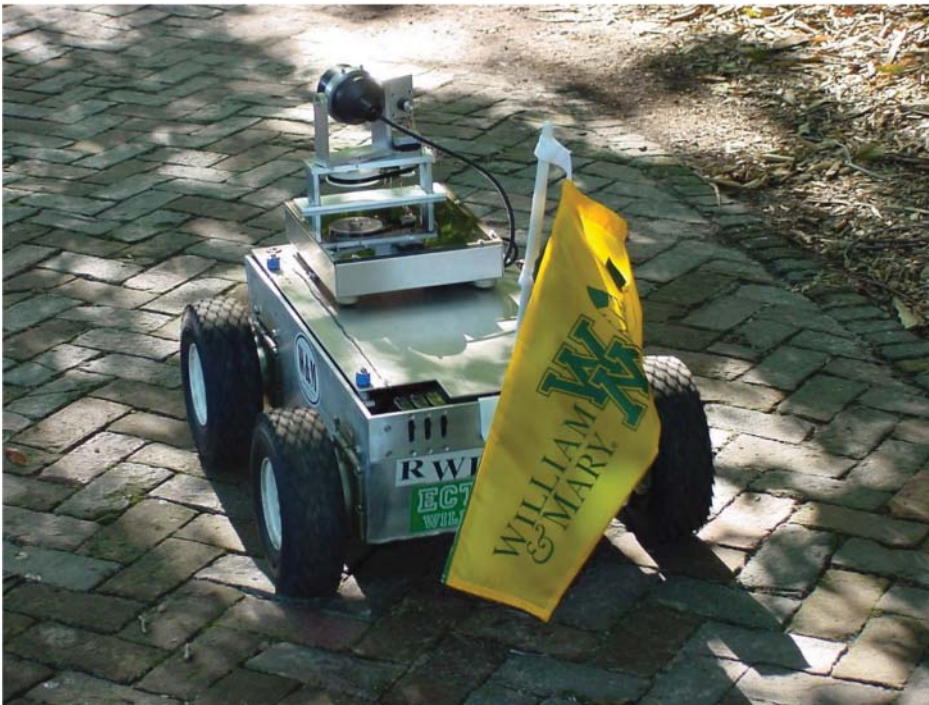
Figure 7.7 A mobile robot which we named rWilliam has a forward-looking 50 kHz pulse-echo scanner mounted in front. As the ultrasound beam sweeps across an upright cylindrical scatterer, the backscatter vs. angle will be symmetric near the peak for a round metal light pole, whereas the bark on a tree will introduce asymmetry into the backscattering because the roughness of the bark is similar in size to the wavelength of sound in air at 50 kHz. Such features can also be used to distinguish big trees from small trees based on backscattering [11] because even so-called “narrow beam” transducers have beams that are too divergent to image in the manner that is done for medical ultrasound.
