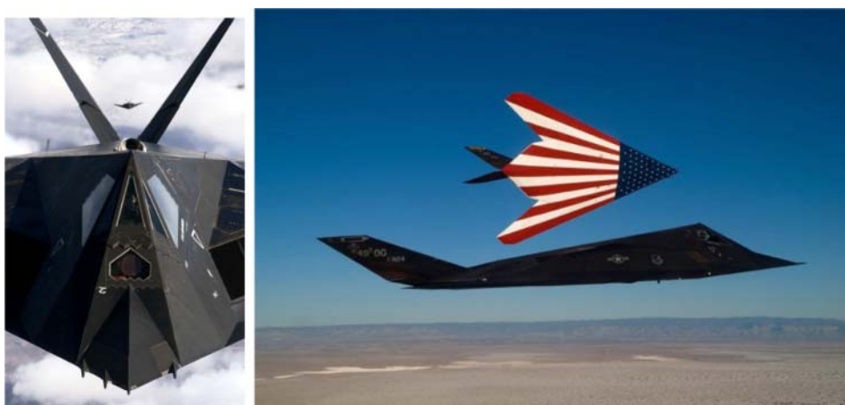
Figure 1.19 Most people first became aware of stealth aircraft when the F117A Nighthawk was used to great effect in Iraq in 1991. The faceted shape is designed to redirect radar, not absorb it. Source: (a) Master Sgt. Lance Cheung/U.S. Air Force/Wikimedia Commons/Public domain. (b) Senior Master Sgt. Kim Frey/U.S. Air Force/Wikimedia Commons/Public domain.
