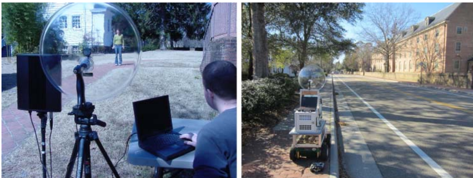
Figure 1.24 Waveform synthesized via Matlab on laptop and sent via headphone jack to parametric array which transmits it via nonlinear ultrasonics. Dish collects back-scattered sound from target and sends it to laptop via microphone jack where Matlab records the digitized waveform for analysis.
