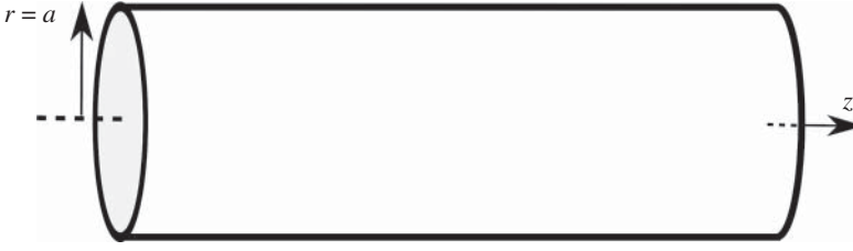
Figure 5.6 Cylindrical rod of radius r = a with propagation in the z -direction.
