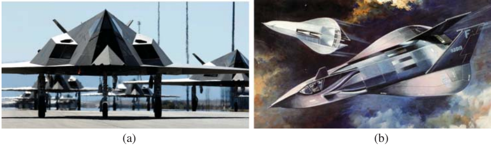
Figure 9.4 Front view of the F117 stealth fighter (a) from which you can see that there are lots of corners and edges where simple GO approaches are going to break down. The facets will be fine, but corners and edges will cause diffraction. Based on what it purported to be “inside” information, Testors released this conceptual F-19 in 1986 (b). Garnering massive media attention, the design became the shape of the mysterious Stealth Fighter in the public’s mind until the actual Stealth – the F-117 Nighthawk – was unveiled in 1990. As it turned out, Testors’ sleek and low-profile Stealth looked not a thing like a highly angular, faceted F-117 it was meant to portray. Source: U.S Air Force/Public Domain.
