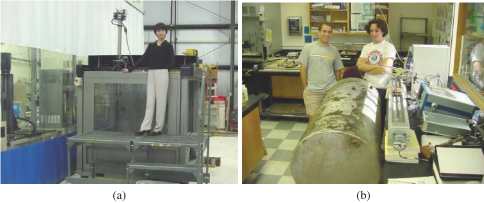
Figure 1.5 Immersion tanks can be quite large, as in this one (a), which holds 6 \times 6 \times 6 -feet of water. Note a smaller tank that holds 2 \times 2 \times 3 -feet of water at the lower left of the image behind the window. In acoustic microscopy where very high frequencies are used to find tiny flaws in small samples, an immersion tank may be a small water container on a high-precision scanning bridge atop a vibration-isolation table. Ultrasound can also be done in contact mode (b), either with hand-held transducers or with scanners configured to have the transducer(s) follow any curvature of the surface.
