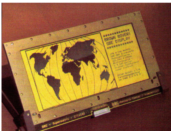
Fig. 1.16 Pioneering super twisted Nematic display
