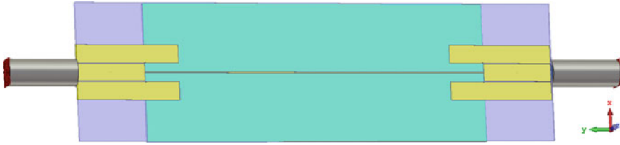
Fig. 7.2 0.05 mm Liquid crystal microstrip phase shifter
