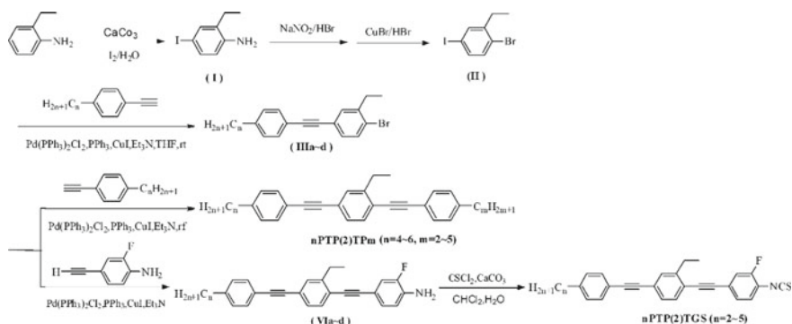
Fig. 4.8 Synthetic route of compounds nPTP(2)TPm and nPTP(2)TGS
