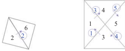
Figure 6.22 Example of mesh to describe the charge density compensation; in black the cell indices, in blue with circles the level-0 function indices
