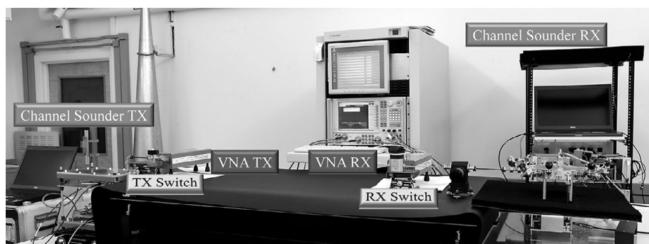
Figure 4.22 Comparison-to-reference 83-GHz channel sounder verification for an LoS propagation channel. A rubber sheet covers the measurement surface. © 2021 IEEE. Reprinted, with permission, from [41].
