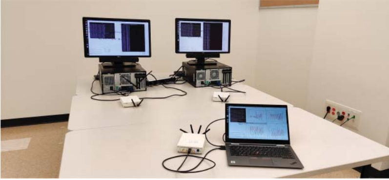
Figure 6.14 GR-WiFi MU-MIMO testbed with 1 AP (laptop) and two STAs (desktops) where real channel response is shown at the AP side.
