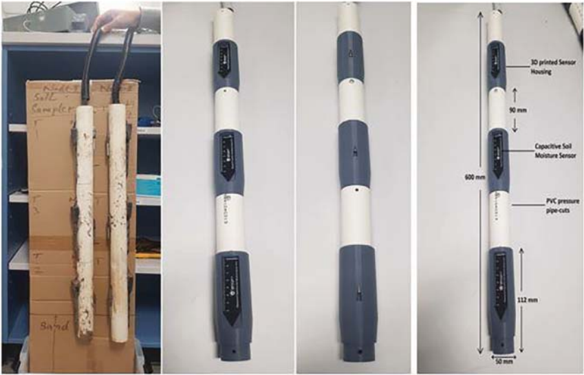
Figure 14.2 Development of a low-cost sensor for monitoring underground soil moisture and soil temperature. Source: Afridi et al. [2023]/IEEE.
