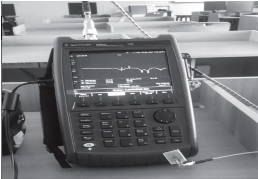
FIGURE 1.7 Fabricated antenna connected to vector network analyzer.
