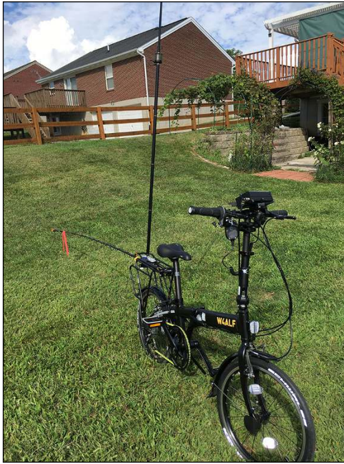
FIGURE 15-2: This folding bicycle-mobile station was built by Christian Bravo, W4ALF, to operate on the HF bands.
