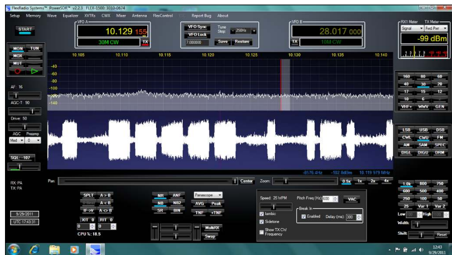
FIGURE 14-1: The PowerSDR software’s operator interface showing a received CW signal along with all of the operating settings and controls.
