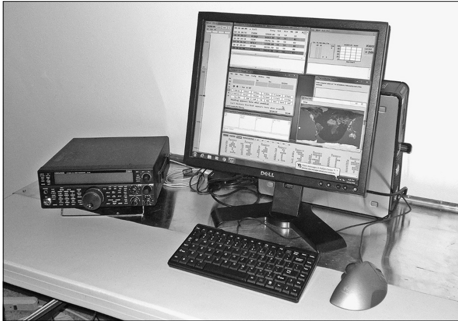
FIGURE 13-9: Metal sheeting under equipment helps control RF picked up from your transmitted signal.
