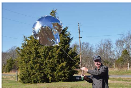
FIGURE 11-4: The WB8ELK Skytracker balloon tracked via APRS.
