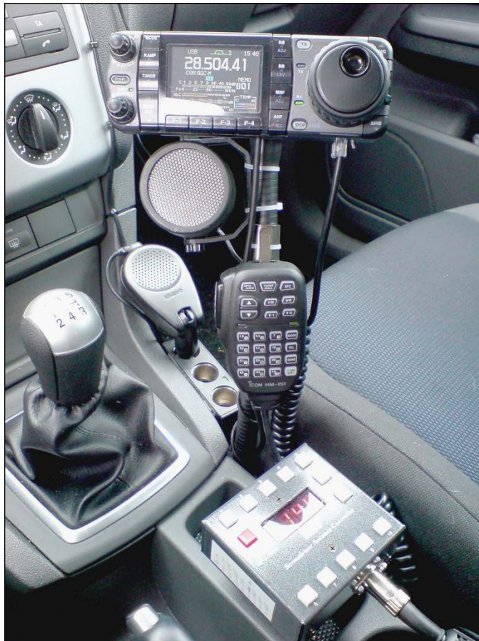
FIGURE 15-3: Most mobile radios have detachable lightweight control heads or faceplates that are easy to secure on flexible or dashboard mounts.
