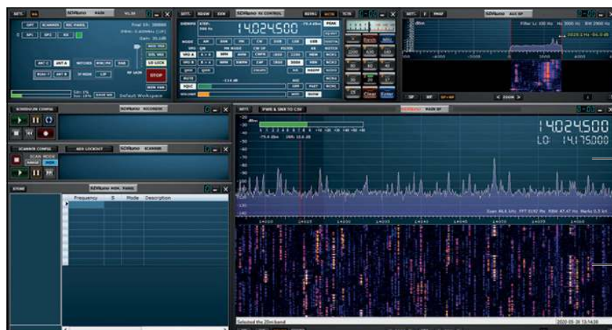
FIGURE 8-4: The SDRuno receiving software simultaneously showing several 20 meter signals on a spectrum and waterfall display at the lower right.
