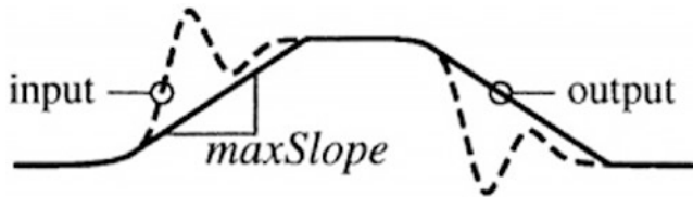
Figure 14-3. Slew filter input-output transformation
