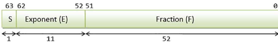
Figure 2-1. The storage format for a 64-bit real type in Verilog-A
