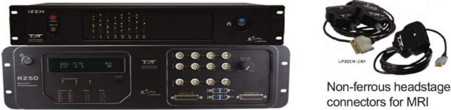
Fig. 4.14 IZ2M stimulator with RZ5D processor base station (left) and MR-compatible non-ferrous headstage connectors (right)
