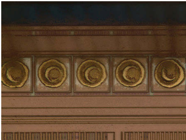
Figure 4.16: Corrosion on bond pads. The brown areas in the bond pad squares are where the Al has been etched away. Image by EAG.
