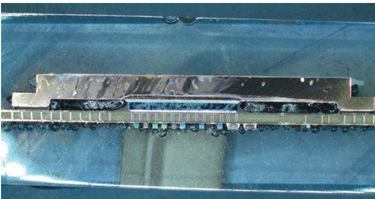
Figure 14.6: A cross section that has residue from improper cleaning. Image by Dan Sullivan.
