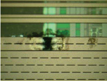
Figure 6.3: Optical image of some Electrical Overstress (EOS) damage in a die. Image by EAG.
