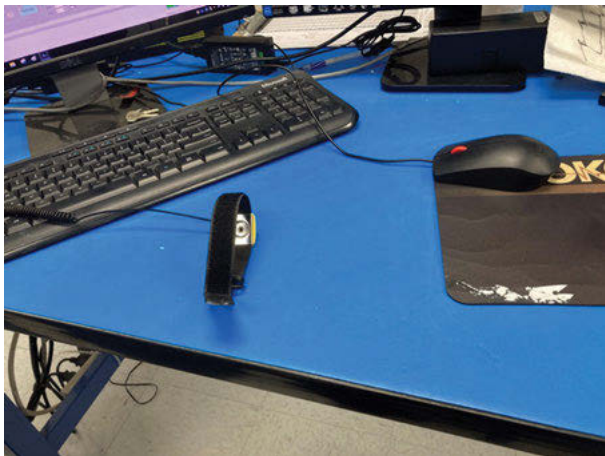
Figure 3.1: ESD work station for a C-SAM tool. Note the blue electrostatic dissipative mat and wrist strap near the keyboard. Image by Dan Sullivan.
