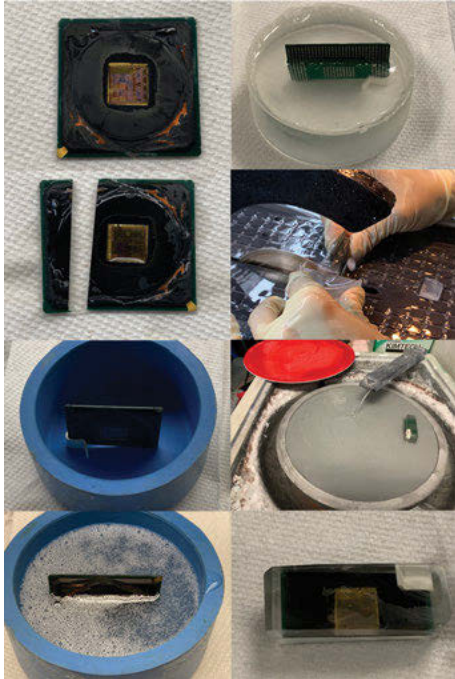
Figure 14.3: Cross section cutting, mounting, and polishing for packaged devices. Process starts with cutting sample to size, mounting, cutting mount to size, and polishing, resulting in final polished cross section mount for further imaging and analysis. Image by Dan Sullivan.
