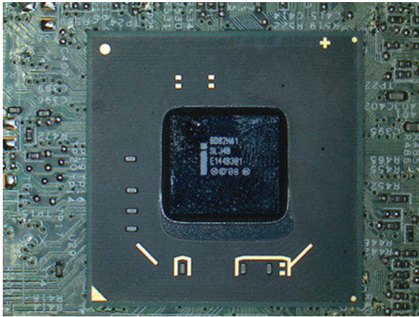
Figure 6.2: As-received device on a PCB. Note that the information on the device in the image allows for retention of information will be lost during the FA process. Image by Dan Sullivan.
