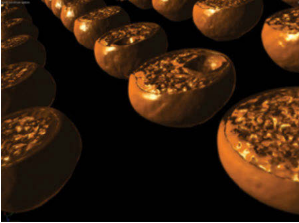
Figure 8.5: Rendered 3D image of solder bumps. Image by EAG.
