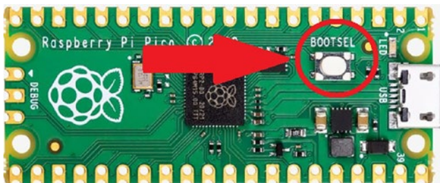
Figure 1-19. Locating the BOOTSEL switch
