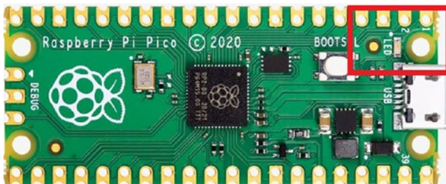
Figure 2-11. Locating the onboard LED (Pico)
