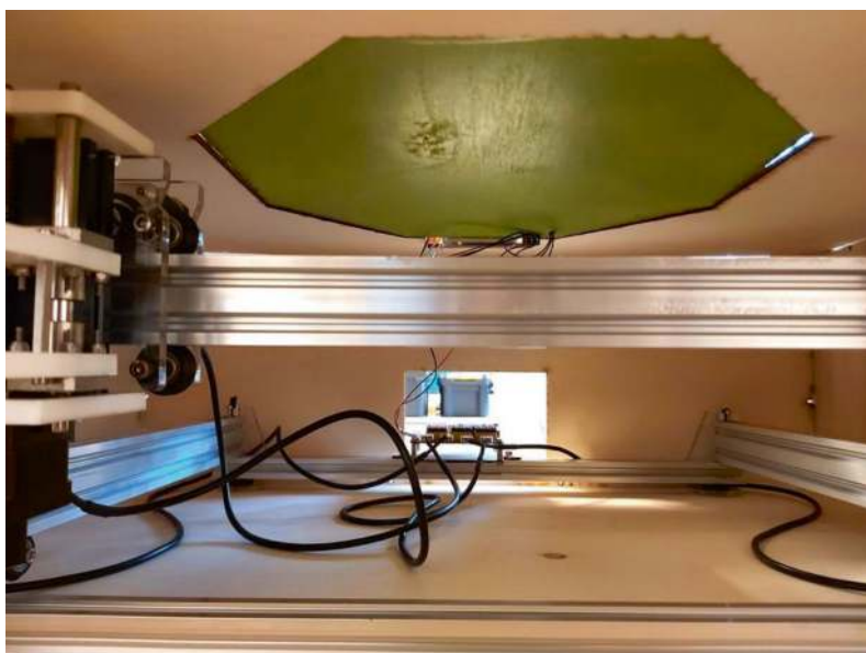
Figure 11-1. Internal view of the moving mechanism upcycled from a CNC structure inside the bottom box of the Sand Machine
