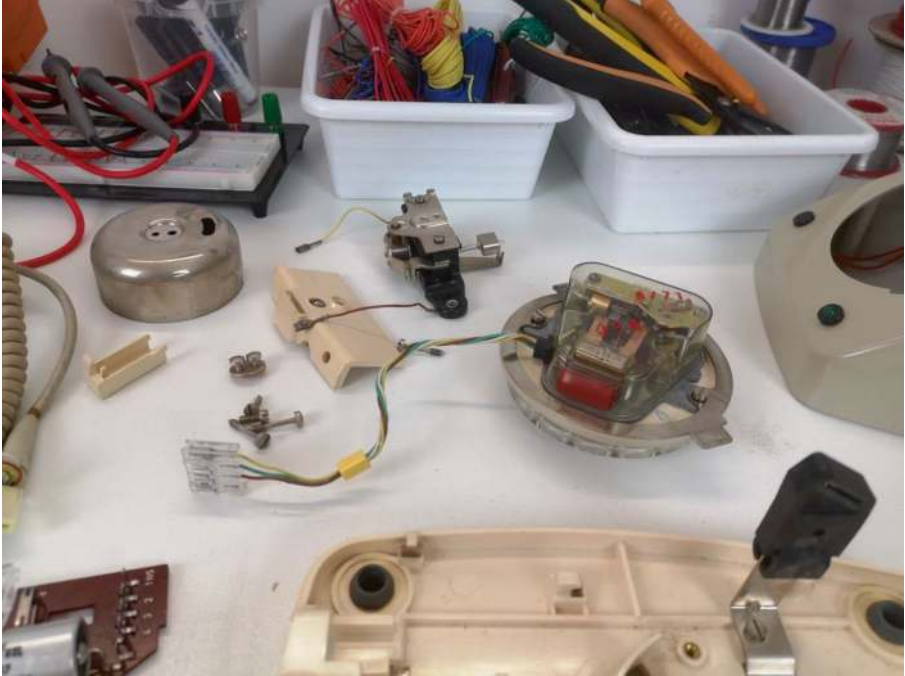
Figure 13-3. I fully disassembled the telephone to understand the space distribution inside the device and how to use some parts. The rotary numbers generator is a relatively modern model, compact and closed inside a plastic box
