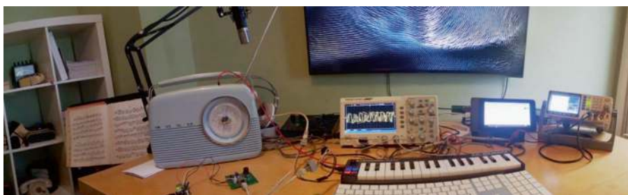
Figure 8-1. The development bench of the Raspberry Pi sound sampler and player. Note that the Radio Magic to the left of the image is used as a noise source, as described in Chapter 17
