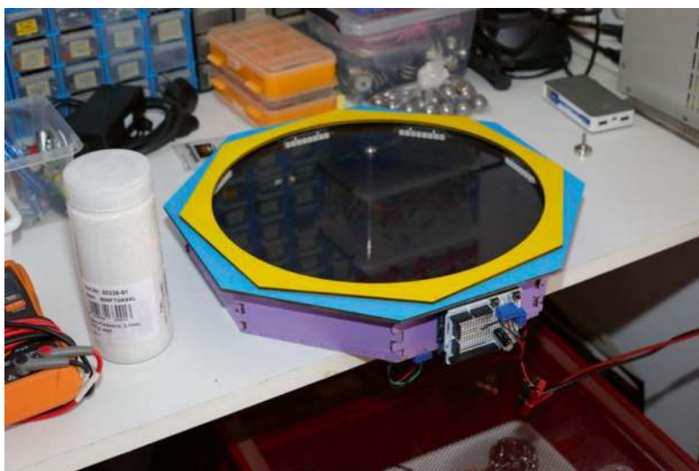
Figure 10-1. The Sand Machine top box was already painted during the final assembly step. Note to the left the first decorative sand used for the first test, which was then replaced with the waterjet calibrated spherical sand
