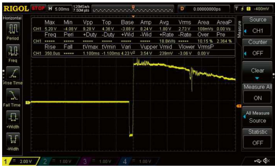
Figure 2-16. The oscilloscope response of the piezo electric sensor ticked with a pen, applying the buffered filter
