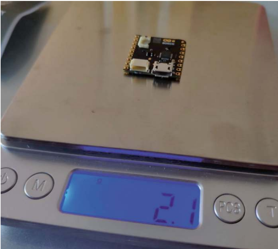
Figure 4-4. The Nicla board only weighs about 2 grams. Including a 3.3V battery, the extra payload is considerably lower than the maximum extra weight the Tello drone can lift off
