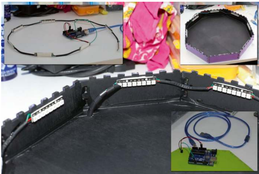
Figure 10-7. Detail of the interiors of the sand dome. The chained Neopixel arrays are distributed on the top of every side of the box, while the three wires (power and control signal) are connected to the Arduino UNO R3 through the bottom of the box
