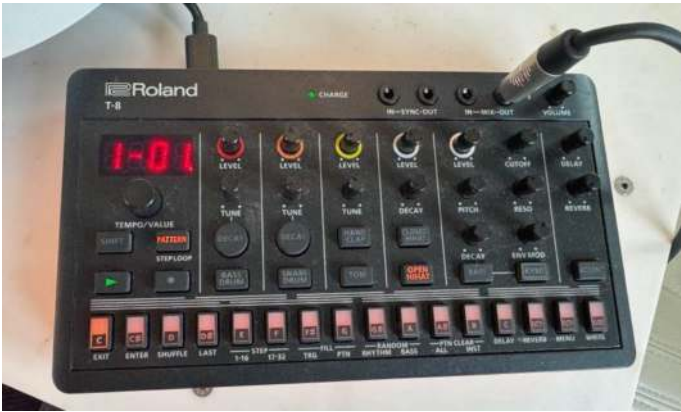
Figure 6-4. This Roland AIRA T-8 is a drum machine that includes the sounds of the iconic TR-606, TR-808, and TR-909 and the bass line sounds of the TB-303. It can be easily connected to a MIDI keyboard and used as the master clock in a chain with other MIDI devices
