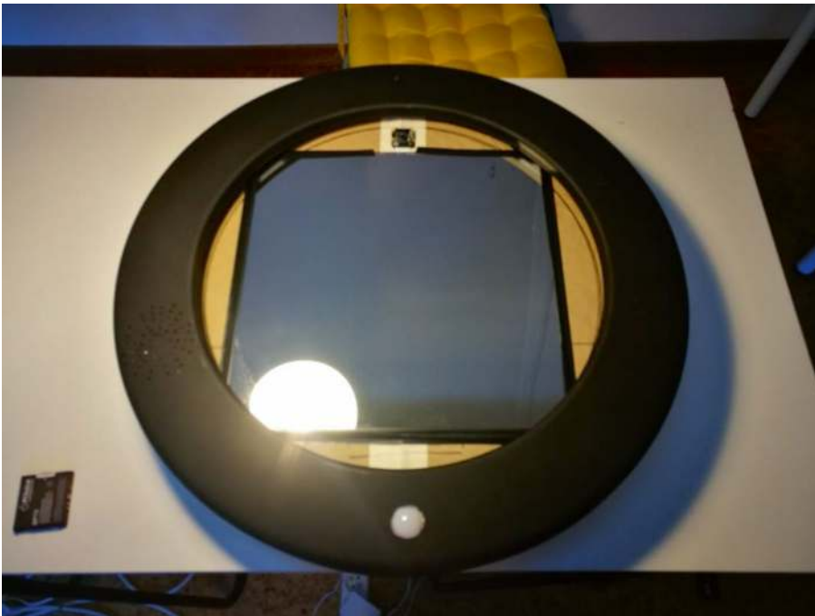
Figure 3-12. The completed assembly of the Scary Mirror. To cover the exposed parts around the mirror and improve the scenographic effect, I hot-glued some black tulle pieces around the device
