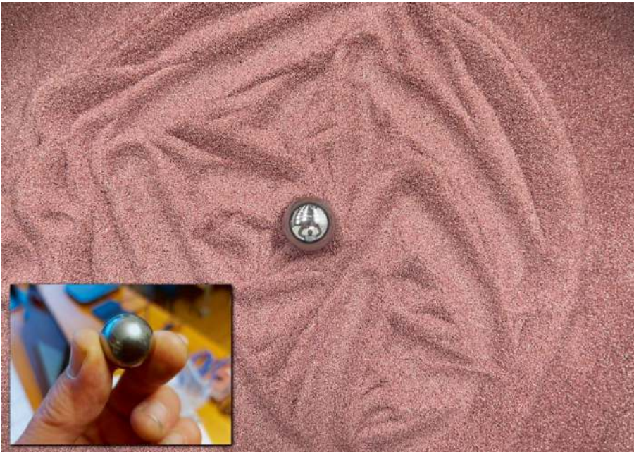
Figure 11-8. Top view of the iron ball (2cm diameter) on the sand dome while testing the movements
