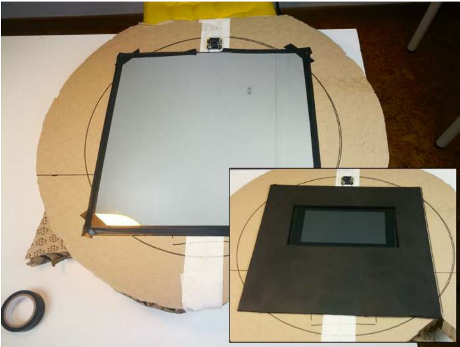
Figure 3-8. The front side of the cardboard block is exposed to the observer's view. The detail shows the Raspberry Pi display with the black cardboard mask to create the perfect reflecting background
