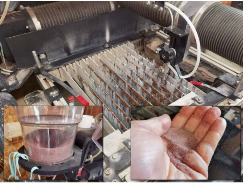
Figure 9-5. The sand used by the waterjet cutter is produced in a spherical shape of 1mm diameter. This artificial sand has the best performance to make the Sand Machine
