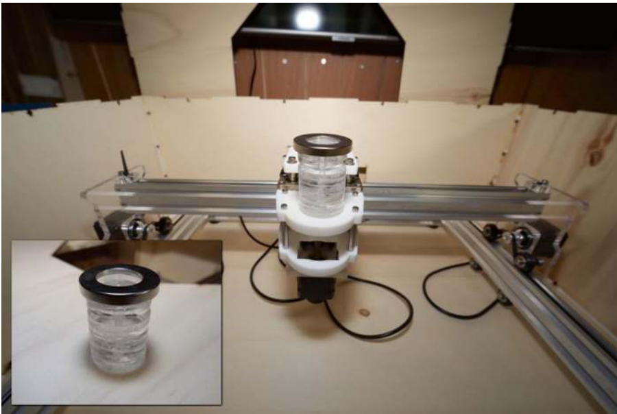
Figure 11-4. Detail of the magnet support on the z-axis head
