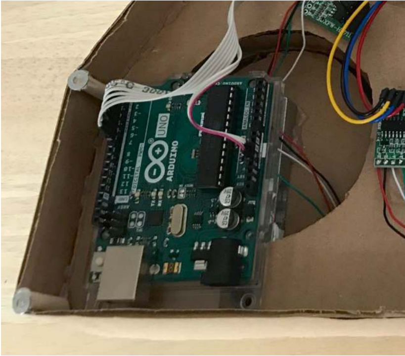
Figure 6-7. Arduino UNO R3 is the core of this project; the microcontroller, with the MIDI library, in this project exposes itself as an electronic musical instrument, sending the notes corresponding to the configured drum instruments
