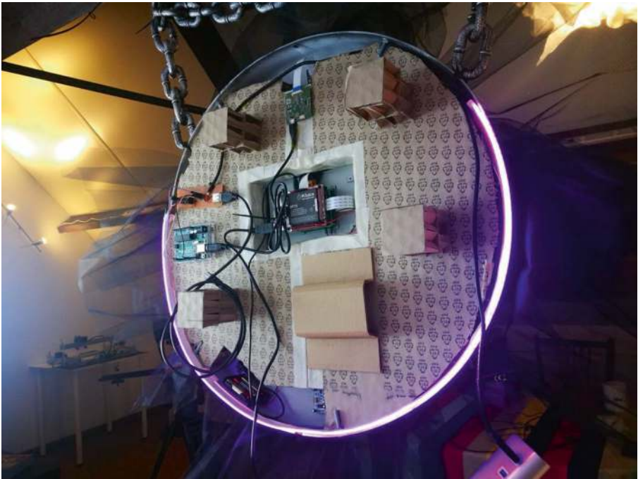
Figure 3-13. The back side of the Scary Mirror. A large portion of the frame circumference holds the 128-Neopixel LED strip. The parts that should be hidden on the front side are covered by a tulle textile
