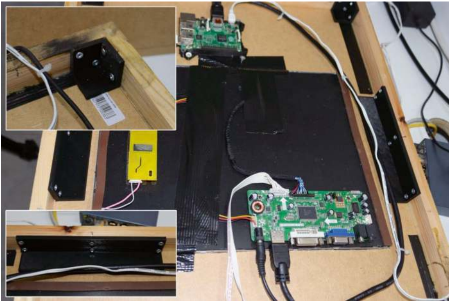
Figure 3-3. The assembled backside of the magic mirror, including the Raspberry Pi and the HDMI screen controller. For this first creation, I followed a very basic setup with the Raspberry Pi running only the MagicMirror2 platform
