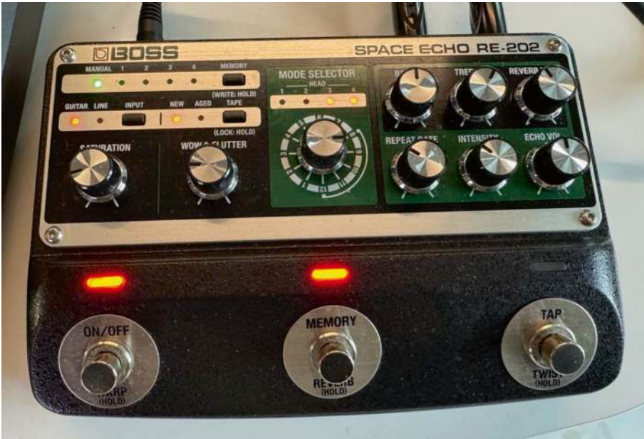
Figure 6-3. This echo effect is the remake of the legendary Boss RE-201 Space Echo, originally using a tape loop, launched by Roland in 1974. This model—able to simulate the same features of its ancestor—includes MIDI-In and MIDI-Out connectors. All the settings are manually accessible by the rotary controls and through MIDI commands
