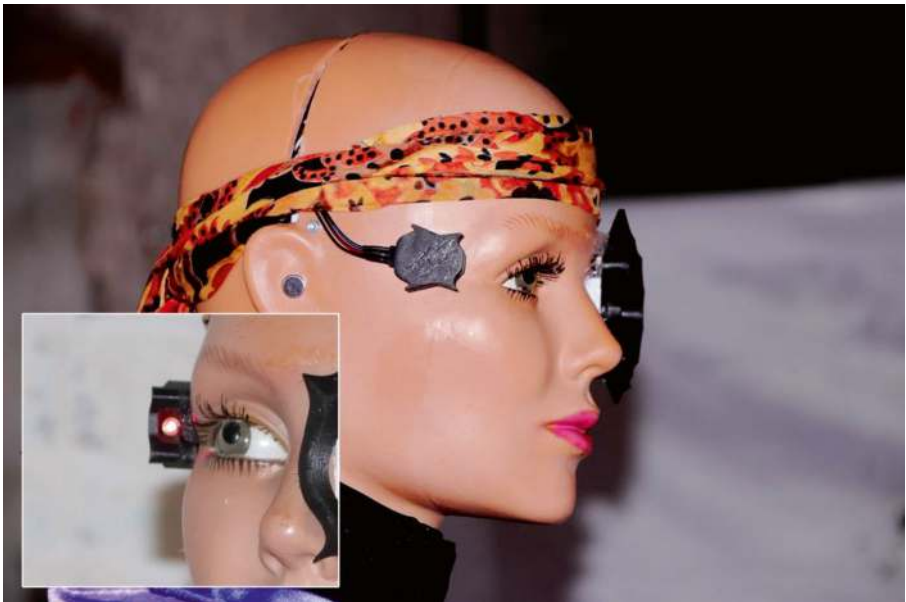
Figure 18-10. The pointing laser was installed on the right side of the face. When armed, it points to the same direction of sight as the right eye
