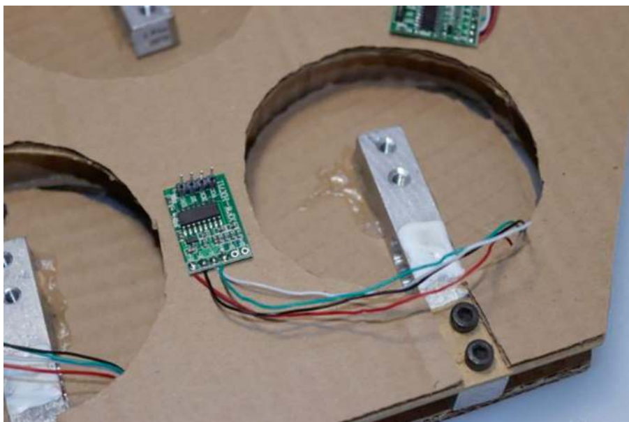
Figure 7-2. Bottom view showing how the load cell is connected to the circular pad. The cell is screwed to the structure of the device and glued to the bottom side of the pad. Any vibration of the pad is transmitted to the load cell
