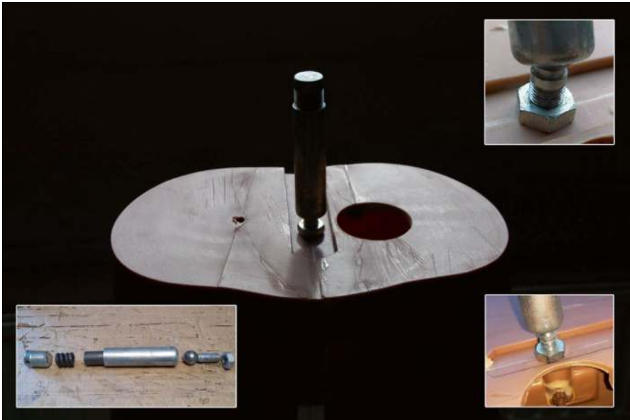
Figure 18-5. The swivel joint is reused to motorize the torso rotation
