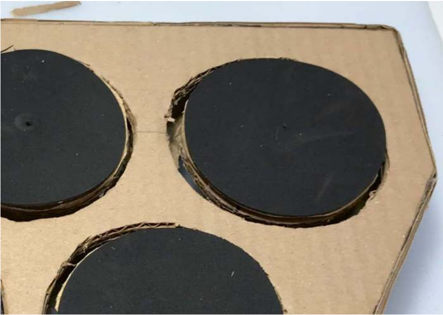
Figure 7-6. Detail of the pads with the top layer composed of a 1mm thick black polyurethane sheet
