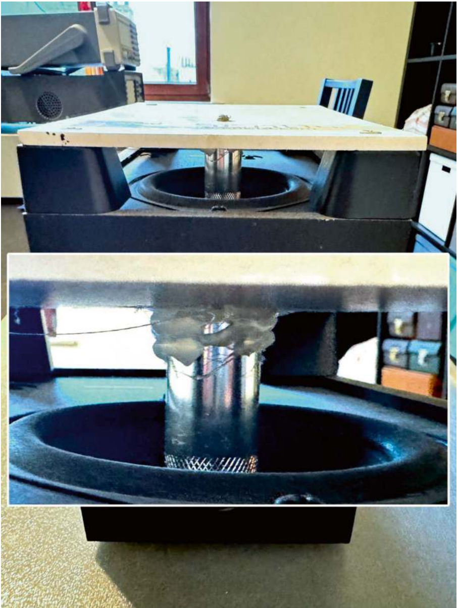
Figure 2-2. Details of the audio subwoofer modified for the vibration platform. The top platform is screwed to the four corners and is connected to the subwoofer speaker through a plastic cylinder, which is glued on both sides
