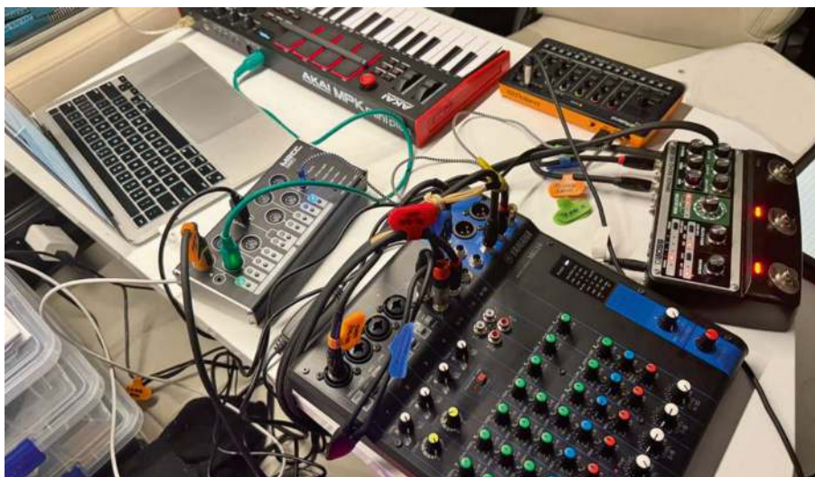
Figure 6-2. Some electronic instruments and effects “chained” together through the MIDI bus. Thanks to the flexibility of MIDI, a small MIDI bus allows you to send the same MIDI message from a source to multiple sources. Indeed, one of the devices is set as a “master clock” to keep all the others synchronized
