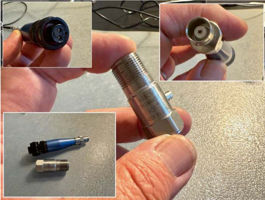
Figure 2-4. The piezo electric vibration sensor for industrial applications used for testing the setup. The sensor (center of image) is connected to a coaxial cable for signal detection, while the opposite side is firmly bolted to the vibration platform
