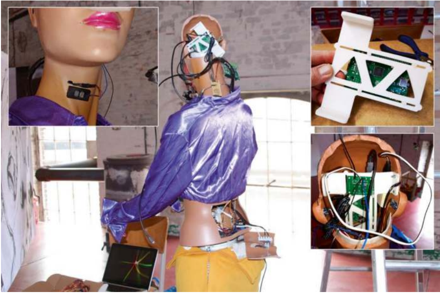
Figure 18-12. The Raspberry Pi installation in the Borg’s head was achieved by 3D-printing flexible support to keep the embedded Linux board in place. The Raspberry Pi controls a small yet powerful speaker glued to the throat
