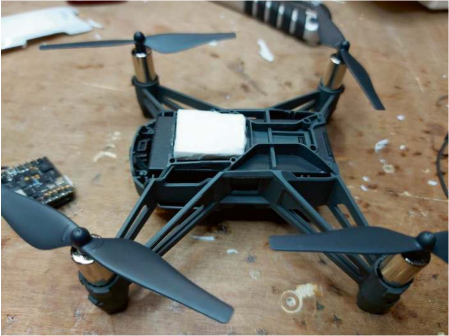
Figure 4-2. The Tello drone's bare metal structure. Removing the plastic cover allows the drone to fly with an extra payload of up to 50g without losing movement stability. To test the payload, I added a small weight (white piece) to reach 50g of extra weight
