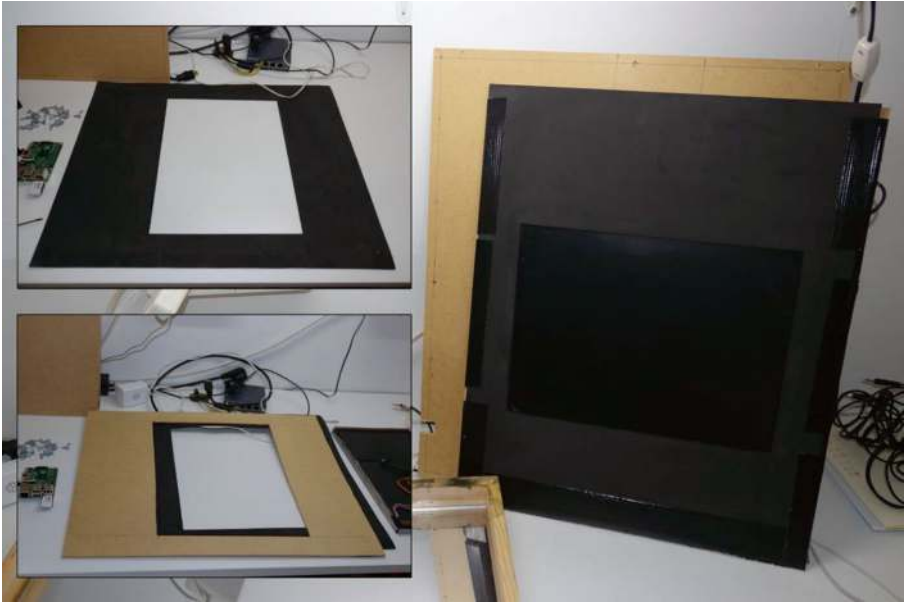
Figure 3-4. The mask components of the back of the mirror create the scenery effect
