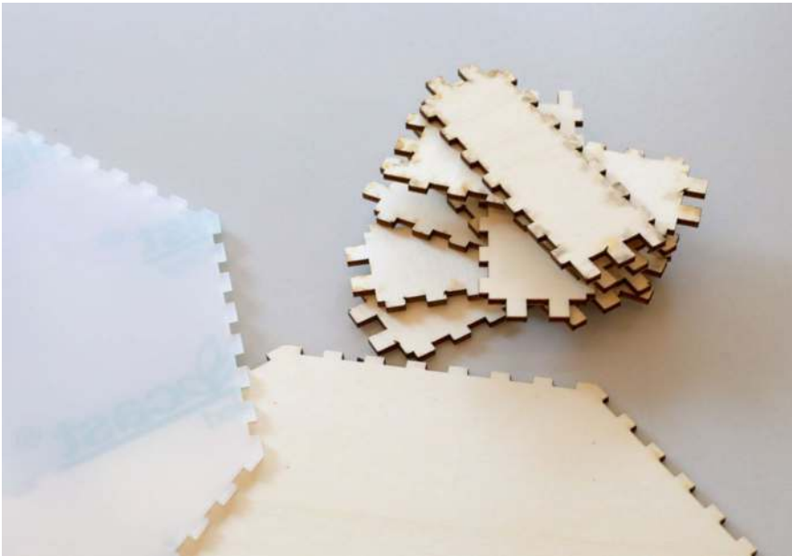
Figure 9-9. A detail of some components after laser-cutting, ready for assembly
