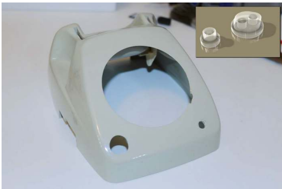
Figure 13-12. The front side of the telephone cover case has two holes to host the status LEDs. The LEDs are covered by cover elements 3D printed with transparent resin
