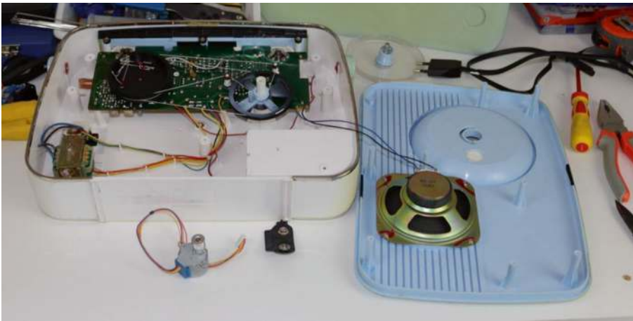
Figure 17-3. The internal body of the radio is disassembled, removing the speaker. This makes sufficient space inside to host a low-speed stepper motor—and the motor controller—to enable the rotation of the variable capacitor.
