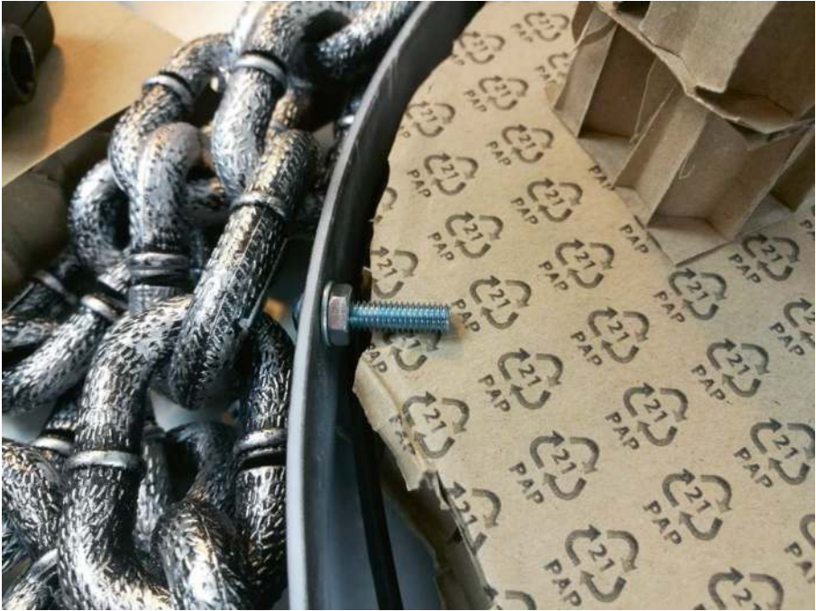
Figure 3-9. Detail of one of the three screws that block the internal build of the Scary Mirror and keep it in place when the mirror is hung vertically
