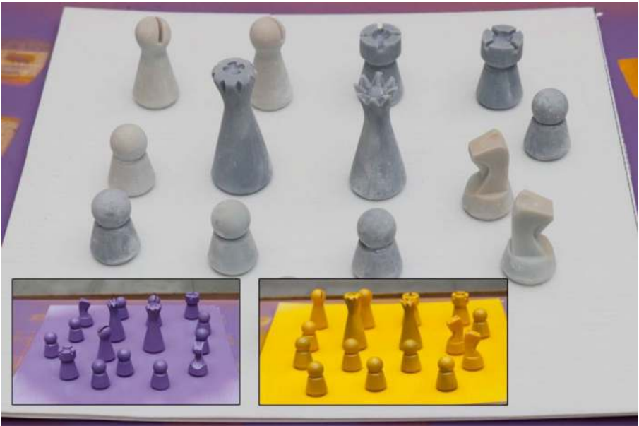
Figure 16-7. The pieces of 3D models were refined and painted with the two opponent colors. To achieve the best quality, I used a high-resolution resin 3D printer.
