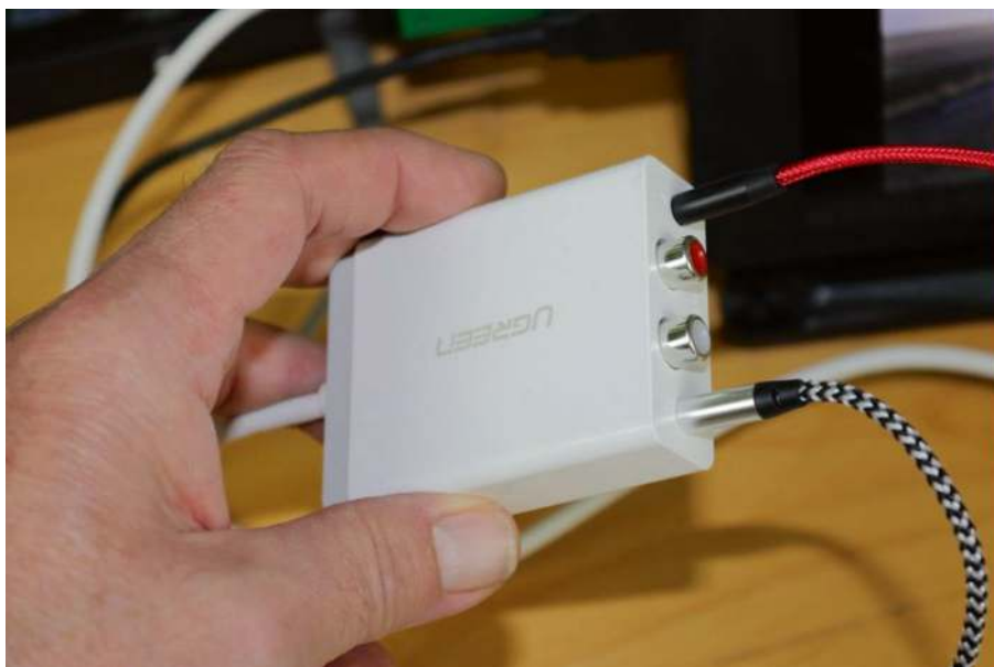
Figure 8-2. One of the USB audio boards I tested on the Raspberry Pi when evaluating the project's feasibility
