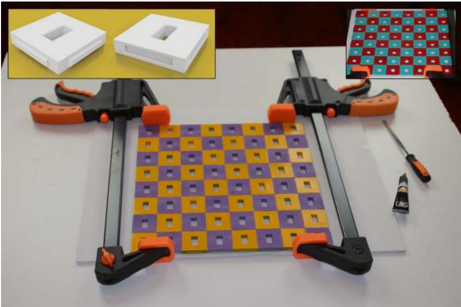
Figure 16-9. The checkerboard tiles were glued after the final assembly. On the top left, the rendering of the tile 3D model shows the opposite sides with the extruded and engraved parts to keep them together. Of course, two identical checkerboards (and two full series of chess pieces) were required for the opponents.
