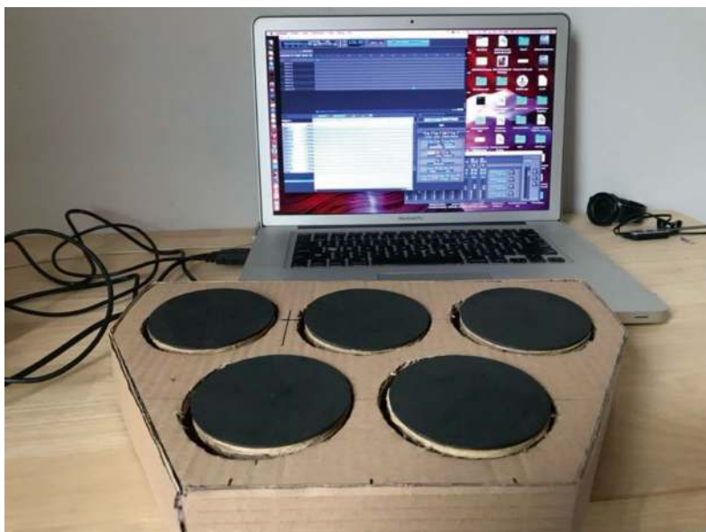
Figure 6-1. The first prototype of the MIDI cardboard drum while recording a rhythm track on my Mac
