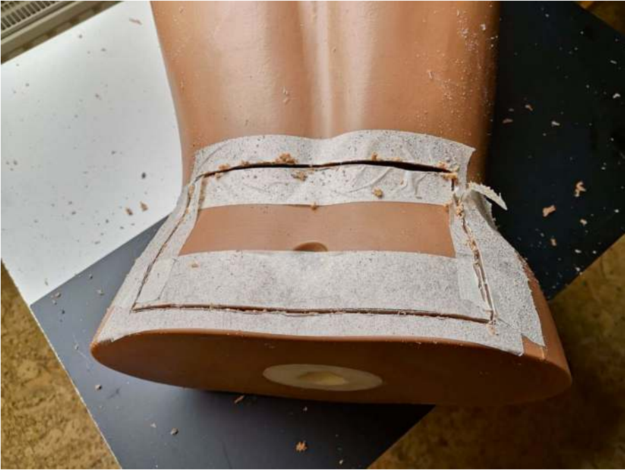
Figure 18-7. The torso opening. I fixed all the components (including the power supplies and wiring) inside this window to control the torso rotation
