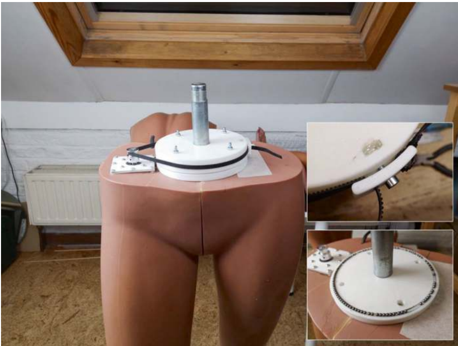
Figure 18-6. The Lazy Susan bearing assembled on the top side of the bottom half of the mannequin
