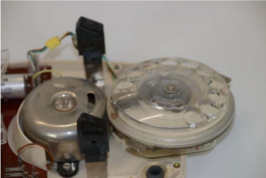
Figure 13-2. The two most important parts of the phone are the rotary dialer and the ring bell. The ring bell became redundant for the project and was removed with the solenoid circuit that excites the bell during an ongoing call
