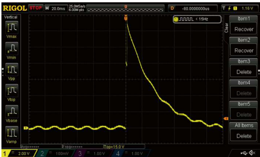
Figure 2-13. With a simple commercial filter, the response of the jellybean piezo, when ticked with a pen, is still too high to avoid the risk of damaging the ADC input
