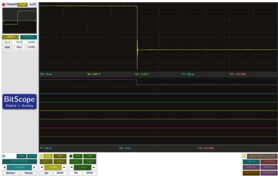
Figure 3-11. The periodic pulse generated by the Arduino UNO GPIO pin is sent to the power bank every five seconds
