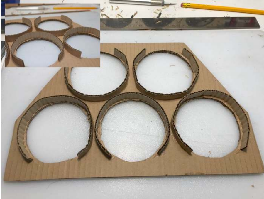
Figure 7-10. Bottom view of the top cover of the drum machine. Around every hole of the pads, there is a cardboard spacer hot-glued to the cover
