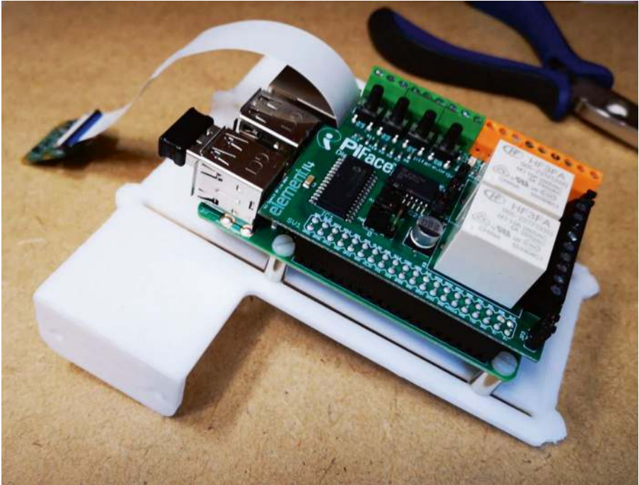
Figure 18-14. The Raspberry Pi with the PiFace digital I/O installed on top and the Pi Camera connected through the flat cable
