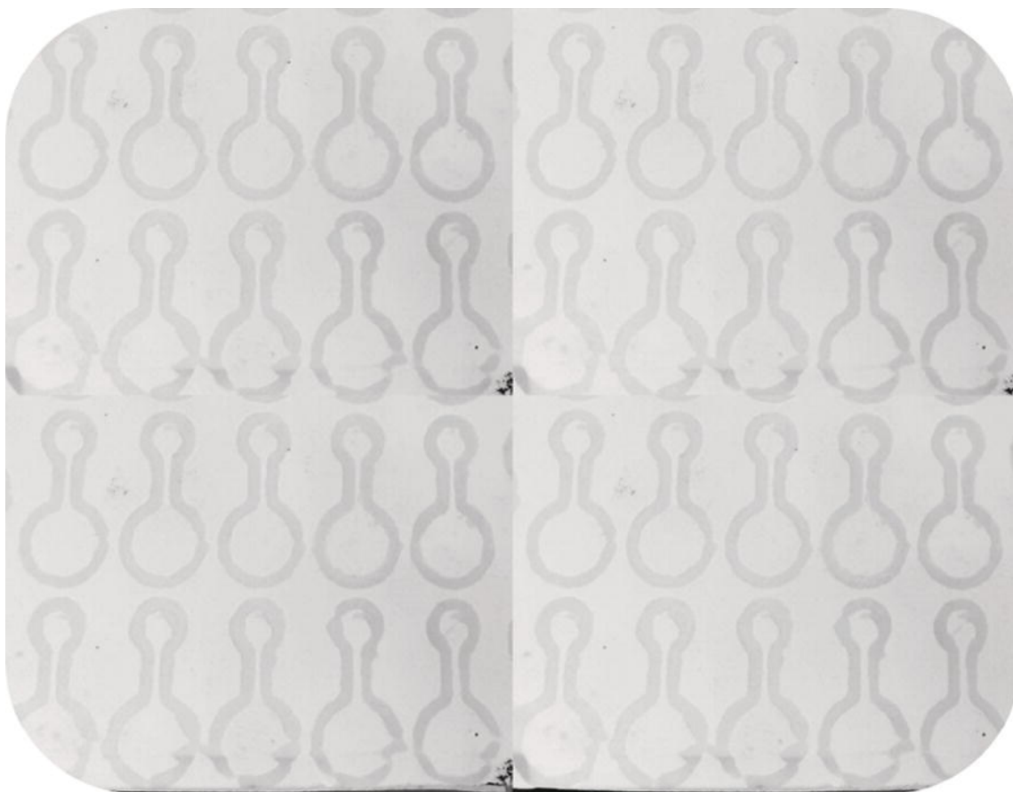
Figure 10.16 3D printed hydrophobic barriers on paper. The traces are of PCL filament, and the region inside the traces would still be hydrophilic.
