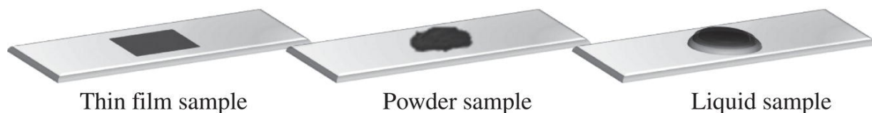
Figure 9.5 Schematic to show the arrangement of the sample on a glass slide for the Raman characterization.
