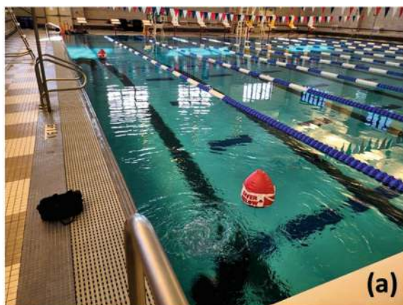
Fig. 4 (a) Photo of an underwater radio communication experiment performed at 50 MHz in pool water (skin depth \eta = 0.1 m). The lateral positions of two divers underwater are marked by two red plastic buoys. (b) Experimental results plotted as communication distance vs. the sum of depths of the two radios underwater. Note that radio communication was achieved over distances of many hundreds of skin depth
