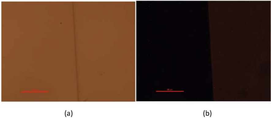
Fig. 14 (a) Reflection microscopic image of an overlap region between 75 nm thick silver film on top of 80 nm thick silver film. The scale bar corresponds to 50 \mu\text{m} . (b) Corresponding transmission image obtained using white light illumination and the same red filter as in Fig. 13c
