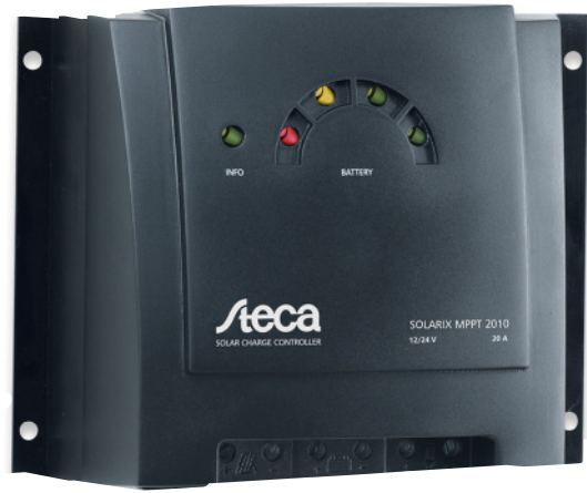
Figure 5.9 This MPPT controller can control a 12 or 24 V system with PV array power up to 500W p and MPP voltages up to 100V. With dimensions 19 × 15 × 7 cm, it weighs 900g (Steca Elektronik GmbH).
