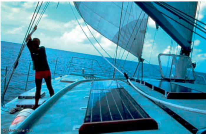
Figure 5.33 It has become commonplace for sailors to install PV modules on the decks of ocean-going yachts to power cabin lighting, services, and navigation equipment. There is now growing interest in making the sails themselves 'photovoltaic' (EPIA/Shell Solar).
