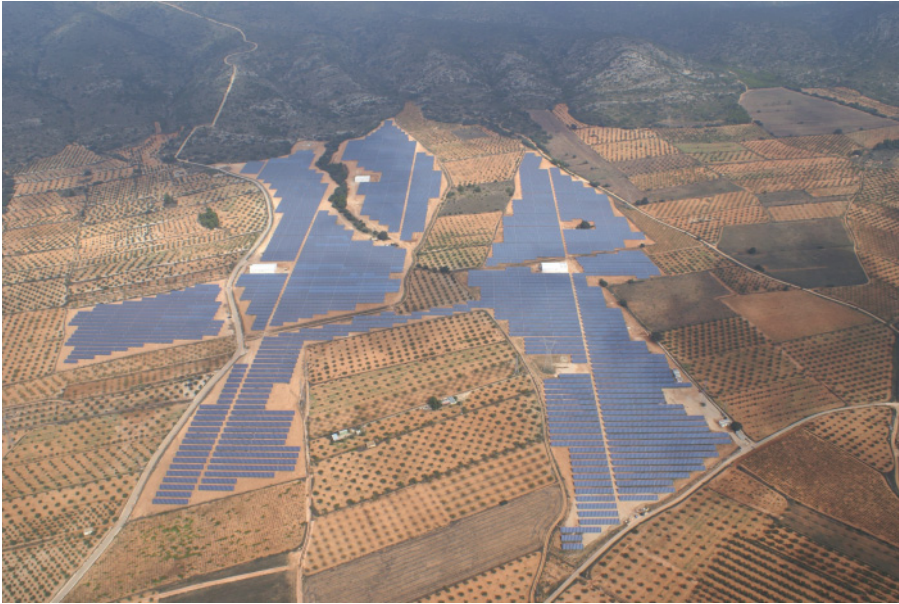
Figure 4.28 A Spanish power plant rated at 1.5\text{MW}_p . This is close to the average size of large PV plants installed internationally by 2008 (IEA-PVPS).
