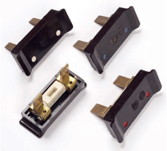
▲ Figure 3.16 A range of BS 3036 rewirable fuses: 5 A (white), 15 A (blue) and 20 A (red)
