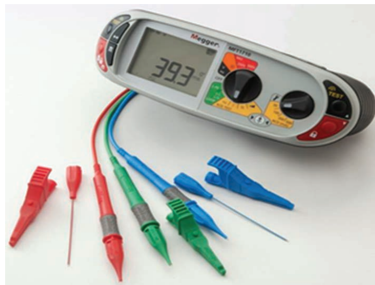
▲ Figure 6.24 Multi-function test instrument showing a range of leads and probes (image courtesy of Megger)
