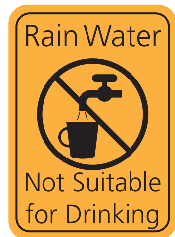
▲ Figure 1.54 Pipework labels that must be fitted
