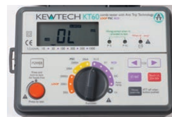
▲ Figure 6.22 RCD testing – this example shows the dial set at RCD – \times \frac{1}{2} with the 30 mA setting displayed in the LCD
