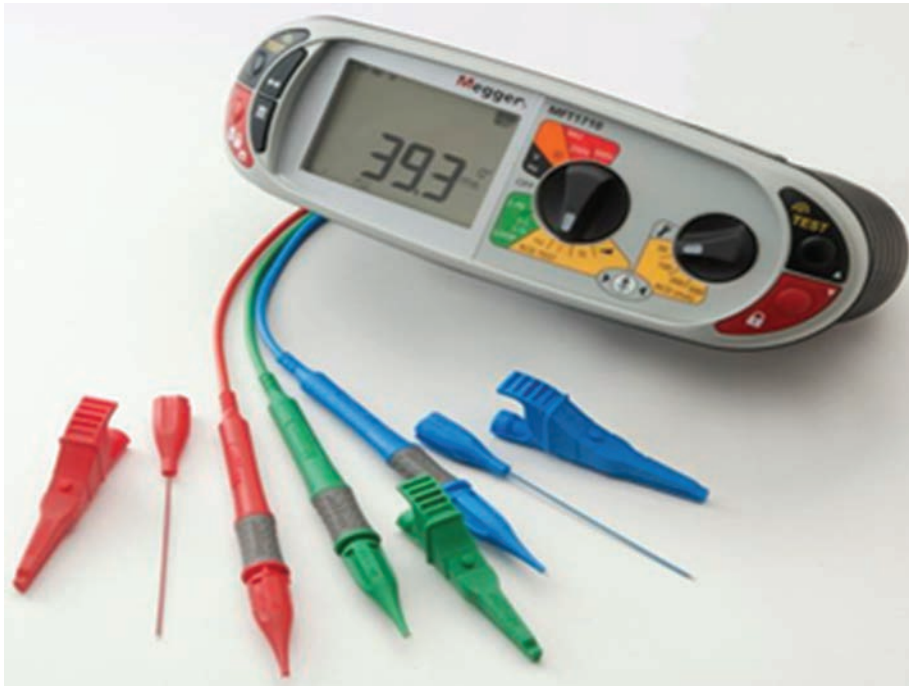
▲ Figure 7.16 Thorough test and inspection at the initial verification stage can minimise faults occurring by picking up installation errors
