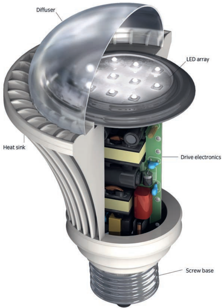
▲ Figure 2.115 Retrofit LED lamp with cut-away showing internal parts
