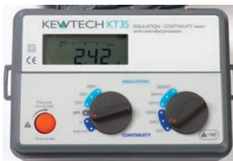
▲ Figure 6.18 Continuity testing – the left dial is set to the \Omega scale and the right dial is set at 20 \Omega
