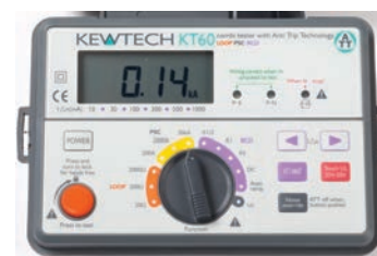
▲ Figure 6.21 Prospective fault current testing – this example shows the dial set at PSC – 20 kA
