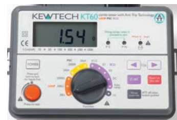
▲ Figure 6.20 Earth fault loop impedance testing – this example shows the dial set at Loop – 20 \Omega . Loop 200 \Omega and 2000 \Omega may need to be used when testing TT systems
