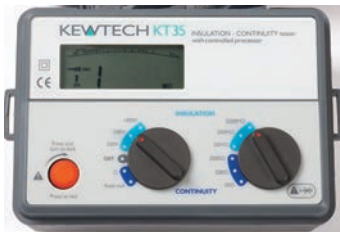
▲ Figure 6.19 Insulation resistance testing – the left dial is set to 500 V and the right dial is set at 2000 M\Omega
