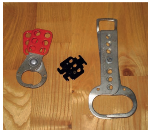
▲ Figure 6.4 Lock-out facility – can be used with one or more locks
