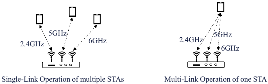
Fig. 3.6 Single-link operation and multi-link operation
