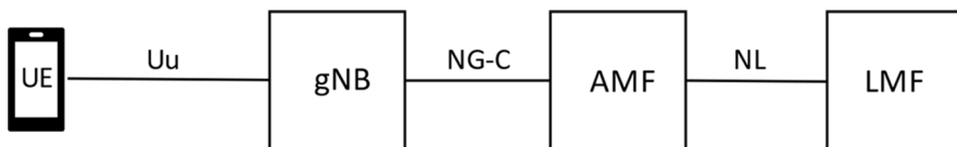
Fig. 8.16 UE positioning architecture applicable to gNB
