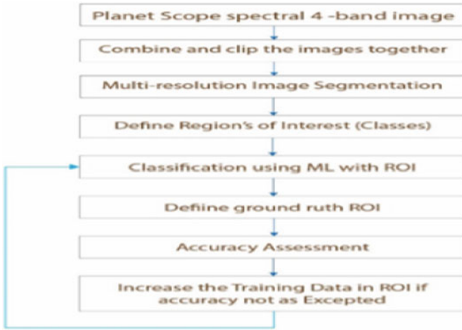
Fig. 2 Flow diagram that shows OBIA and classification workflow
