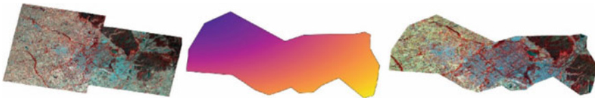
Fig. 3 Pre-process of image shown here uses mosaicking to merge the image and shapefile to clip the image
