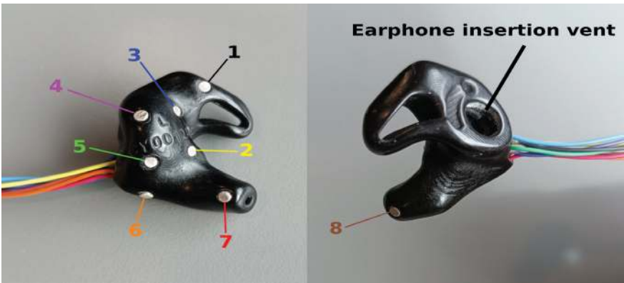
Figure 27. EEG earbuds developed by Segotia. Internal side of the tested earbuds (left). External side of the tested earbuds (right). Sensors are numbered in order of signal channel acquisition 1–8.
