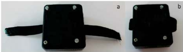
Figure 17. 3D-printed enclosure with elastic straps to fit child’s ankle. (a) Front, (b) Back.
