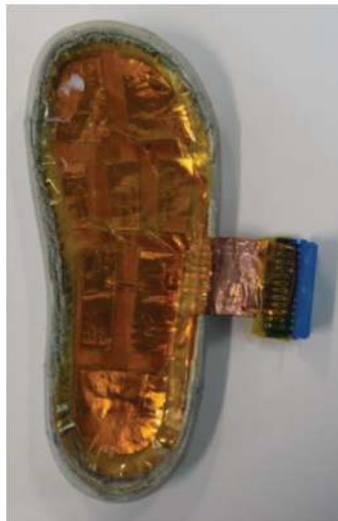
Figure 6. Assembled sensor installed on the outsole.
