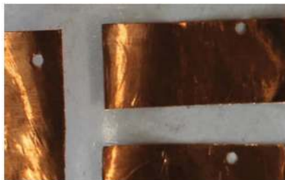
Figure 4. Through holes in the sensor pad for the conductive thread to join with the route layer.
