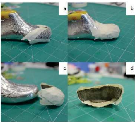
Figure 6. Example of the fabric sensors installed using 80/20 PES/SS sample. (a–c) low tack masking tape is used to shape the fabric sensor insulating the other layer. (d) completed sensor to go inside the toe area of the shoe.
