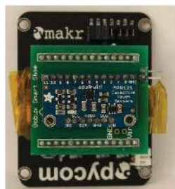
Figure 15. PCB shield assembled on top of the Pycom Expansion Board.
