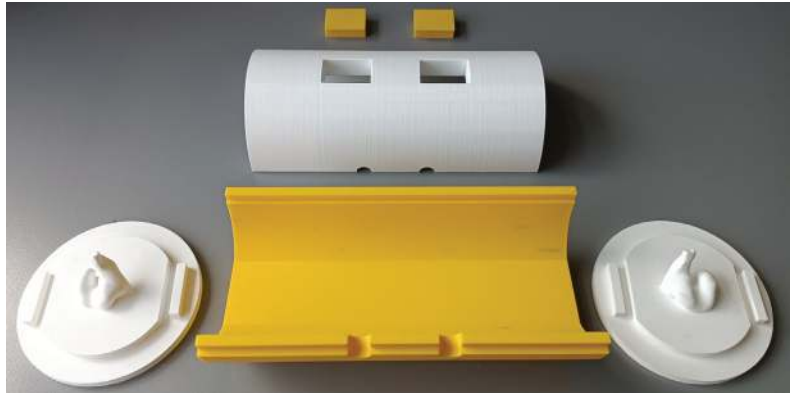
Figure 19. Disassembled ear-EEG phantom: bottom half (yellow), top half (white), and two lids with a left and right ear imprint from one of the test subjects.
