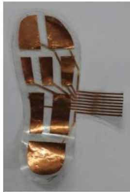
Figure 2. Cut-out of sensor areas using Vinyl Cutter.
