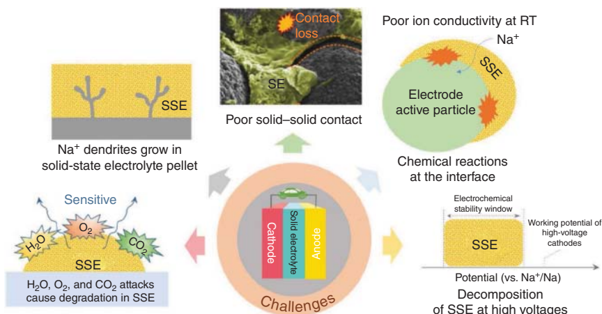
Figure 13.3 Remaining challenges of solid-state electrolytes: (i) unsatisfied ion conductivity at room temperature, (ii) potential Na dendrite growth inside the SSE, (iii) poor solid–solid contact during operation, (iv) high air sensitivity of SSE, (v) unfavorable interactions at the solid–solid interface, and (vi) decomposition of SSE at high voltages. Source: Zhao et al. [8]. Reproduced with permission, 2020, Royal Society of Chemistry.
