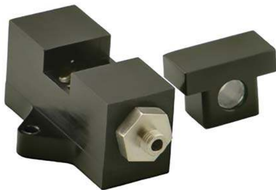
Figure 20.1 The stability monitoring reference cell is installed inside the environmentally controlled analyzer enclosure. Inside the sample holder is a polymeric crystal that provides a repeatable spectral fingerprint. Source: Ryan Lerud / Process Insights-Guided Wave Inc.
