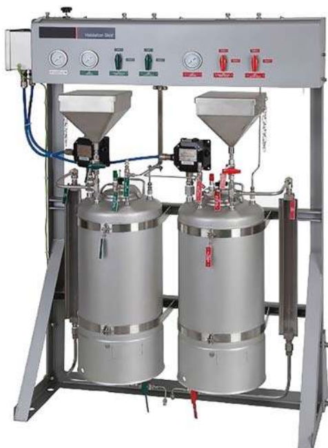
Figure 20.2 Wash and validation skid provides wash solvent (methylcyclohexane) for the sample cells and instrument standardization solvent (spectrophotometric-grade Toluene) for periodic background and validation. Contains a 3–6 month supply of reagent. Source: Author: Ryan Lerud / Process Insights-Guided Wave Inc.
