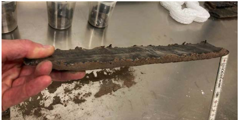
CLOCKWISE FROM TOP LEFT The triangular 'paving stones' interlock to create solid surfaces; how the roads could look; a single melt layer is approximately 2cm deep; melting simulant Moon dust using a carbon-dioxide laser beam
