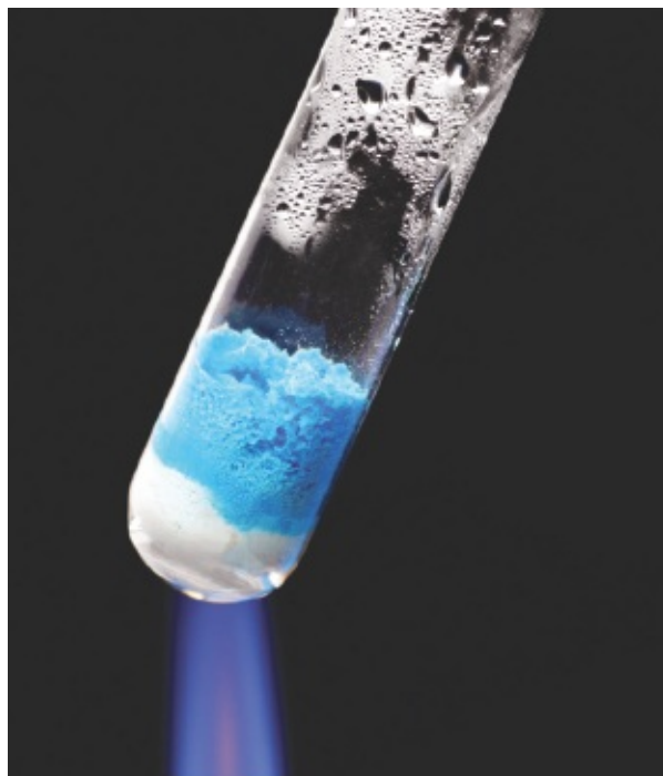
▲ Figure 17.22 Blue hydrated copper(II) sulfate changes to white anhydrous copper(II) sulfate on heating
