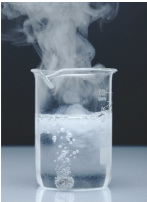
▲ Figure 20.2 A chunk of calcium reacting with water. Notice that it sinks and there are bubbles. A white precipitate of calcium hydroxide forms
