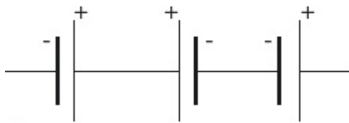
▲ Figure 37.5 Three battery cells in series
