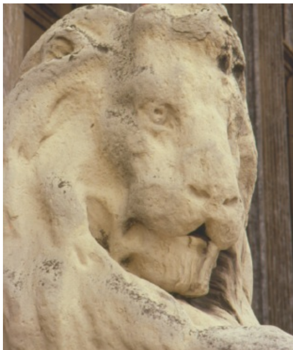
▲ Figure 24.10 This limestone statue outside Leeds Town Hall has been damaged by acid rain
