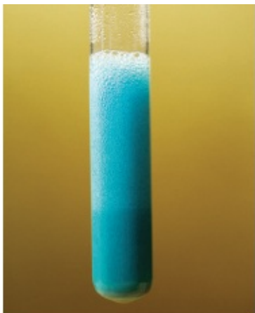
▲ Figure 18.17 Green copper(II) carbonate reacting with sulfuric acid to produce a blue solution of copper(II) sulfate
