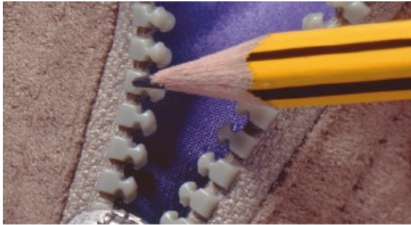
▲ Figure 15.31 Graphite in a pencil being used to lubricate a zip fastener
