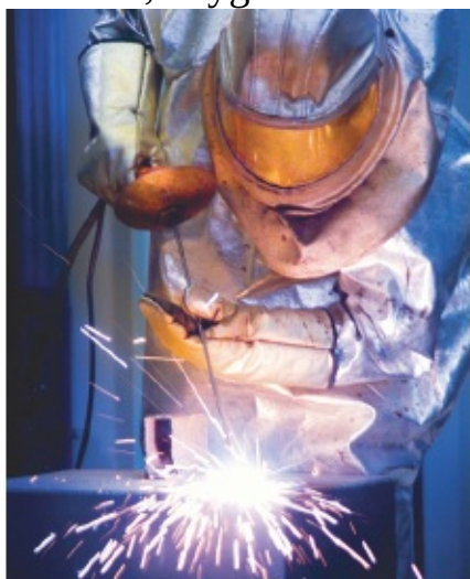
▲ Figure 28.7 A worker using oxyacetylene welding equipment. This equipment burns a mixture of oxygen and acetylene, allowing a flame temperature of about 3300\text{ }^{\circ}\text{C} to be attained
