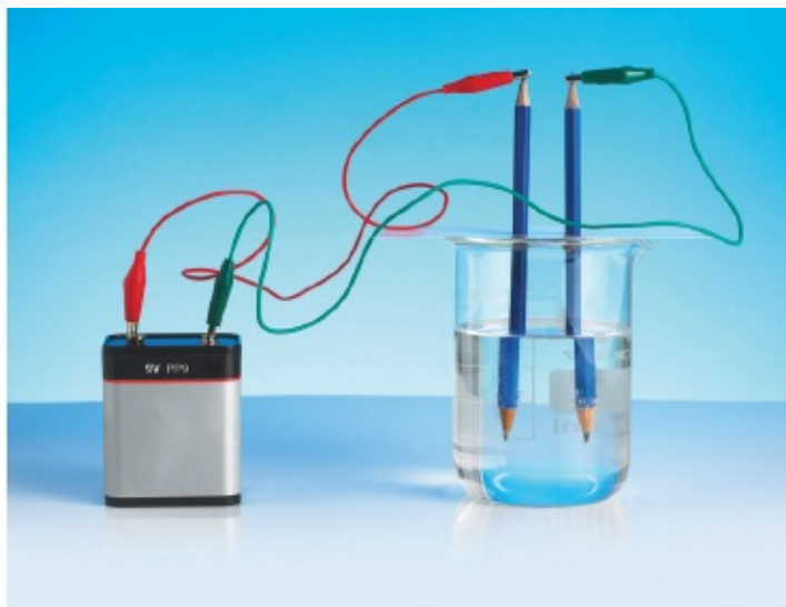
▲ Figure 26.3 The graphite in the 'lead' of pencils is used here to form the electrodes in the electrolysis of water.
