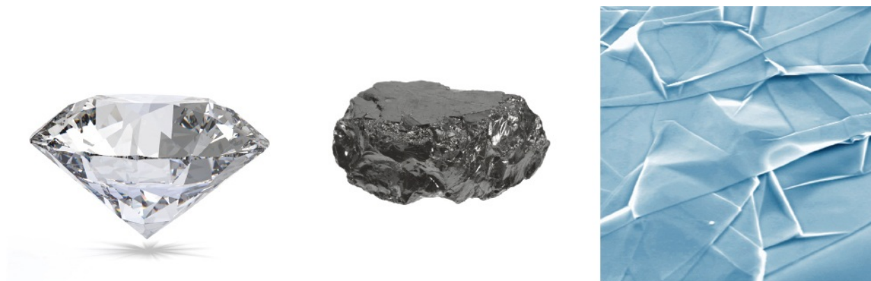
▲ Figure 15.26 Diamond, graphite and graphene are three very different giant covalent substances, but are all composed of the same element. The photo of graphene is an electron micrograph and shows the thin sheets
