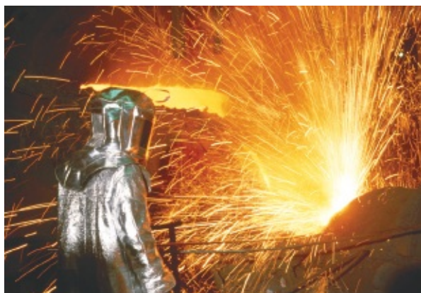
▲ Figure 21.10 A worker in a protective suit beside a stream of molten metal that is pouring from a blast furnace. Heat radiated from the metal is reflected away by the shiny surface of the protective suit
