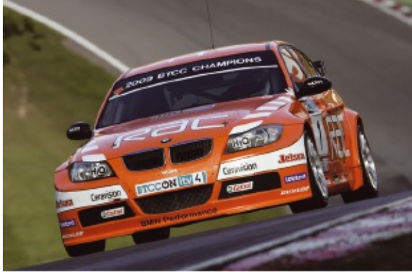
▲ Figure 31.21 This racing car is extremely stable because of its low centre of gravity and wide wheelbase
