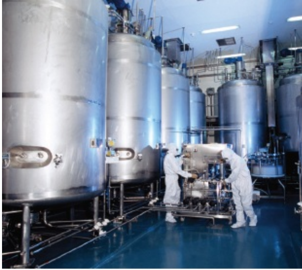
▲ Figure 10.22 Making human insulin by genetic engineering in giant bioreactors (fermenters)
