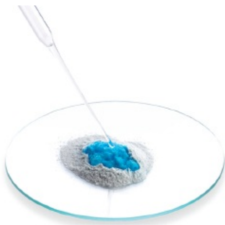
▲ Figure 19.18 White anhydrous copper(II) sulfate turns blue in the presence of water
