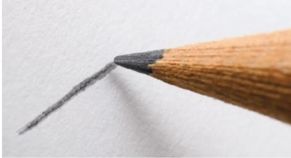
▲ Figure 15.30 Pencil makes a mark on paper because the layers of graphite are only held by weak forces and slip off easily, leaving a mark
