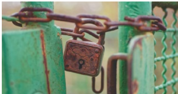
▲ Figure 21.7 An iron padlock rusting. Note that rust is a red-brown flaky substance
