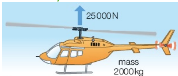
▲ Figure 30.13 Forces acting on a helicopter
