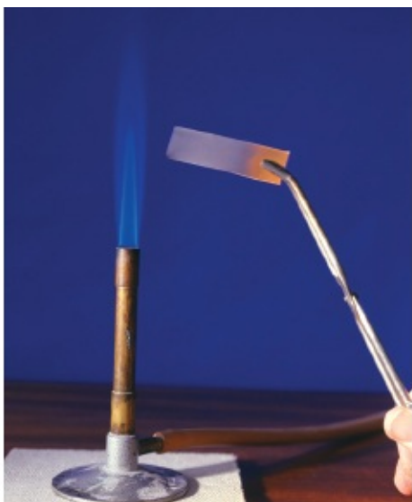
▲ Figure 28.11 Copper being heated in a Bunsen flame. It becomes covered with a black layer
