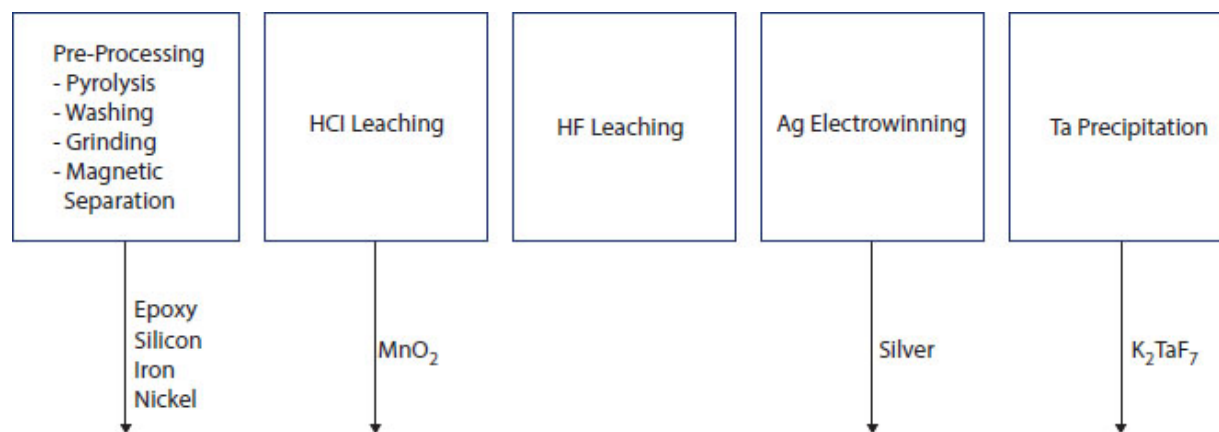
Figure 49.2 Proposed process for Ta recovery from capacitors.
