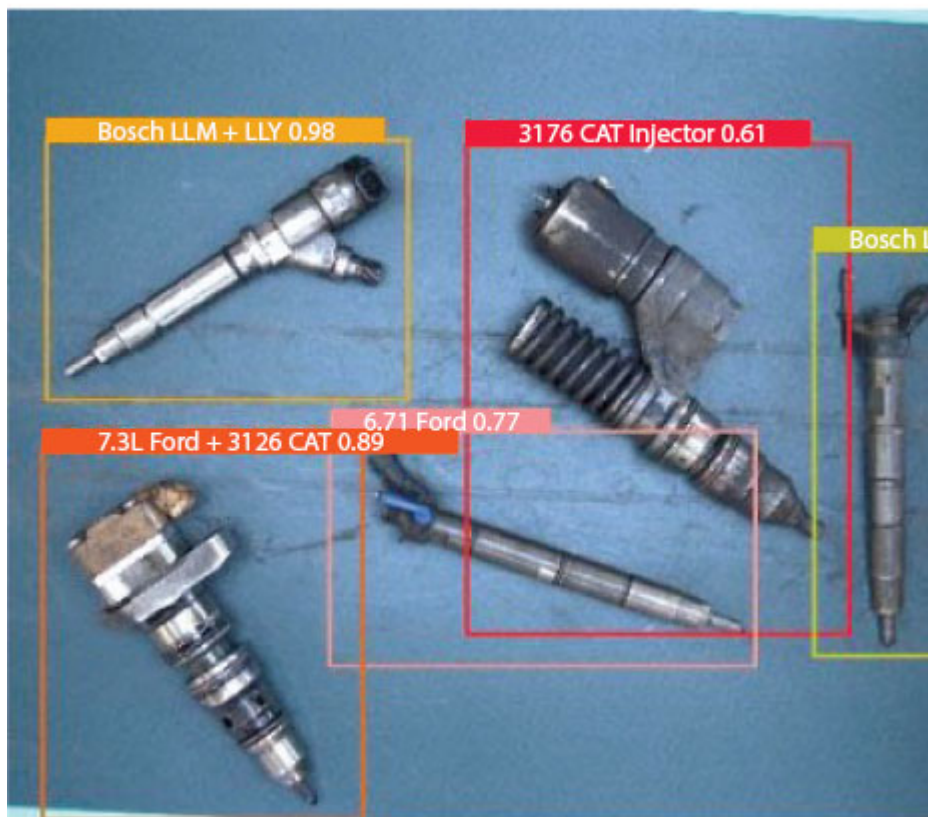
Figure 39.18 Fuel injector detection.
