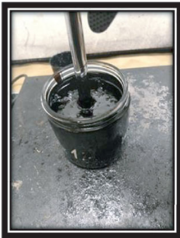
Figure 28.2 Test setup for polymer-modified asphalt.
