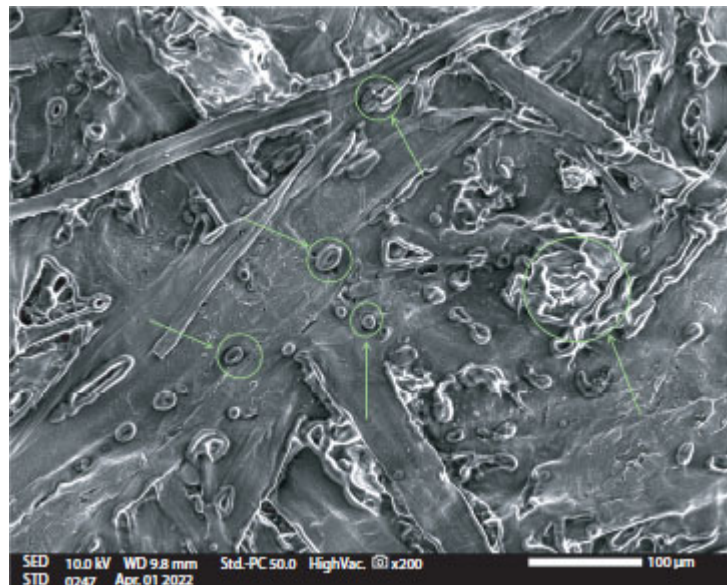
Figure 35.3 SEM images of sticky contaminants on Residential Wastepaper – sticky contaminants in forms of oil droplets and films [19]. (200 times magnification, the scale bar is 100 microns.)
