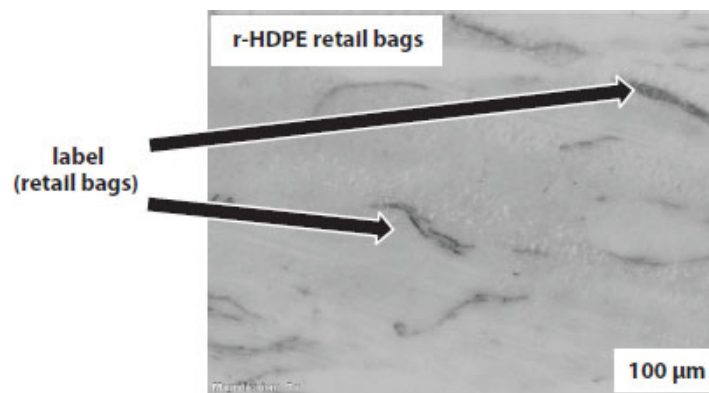
Figure 26.6 Microscopic images from cross-sectional cuts of molded composite from r-HDPE retail bags.
