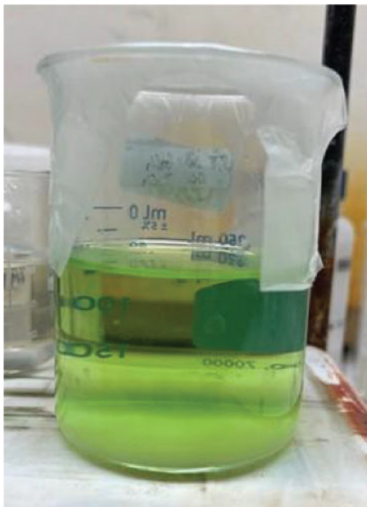
Figure 49.5 Filtered HCl leachate after 3 hours of leaching capacitors.
