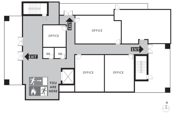
Figure 5.13 Emergency Egress Plan typically found in public view in all buildings of public accommodation which can serve as a starting point for your analysis of the existing building.
