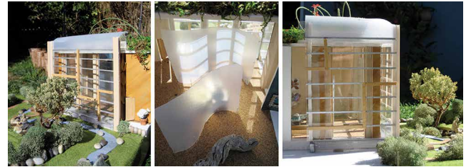
Figure 8.9 Three views of a student’s scale model to study filtering daylight to reduce damage to artwork while still providing the benefits of natural light to museum occupants.
