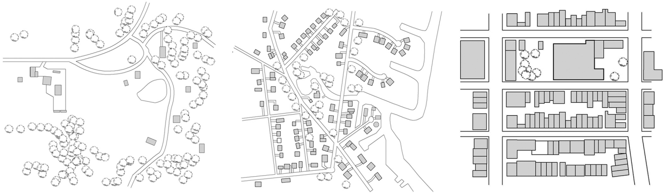
Figure 5.7 Relative population density of the built environment differentiates the building patterns in rural, suburban, and urban regions.
