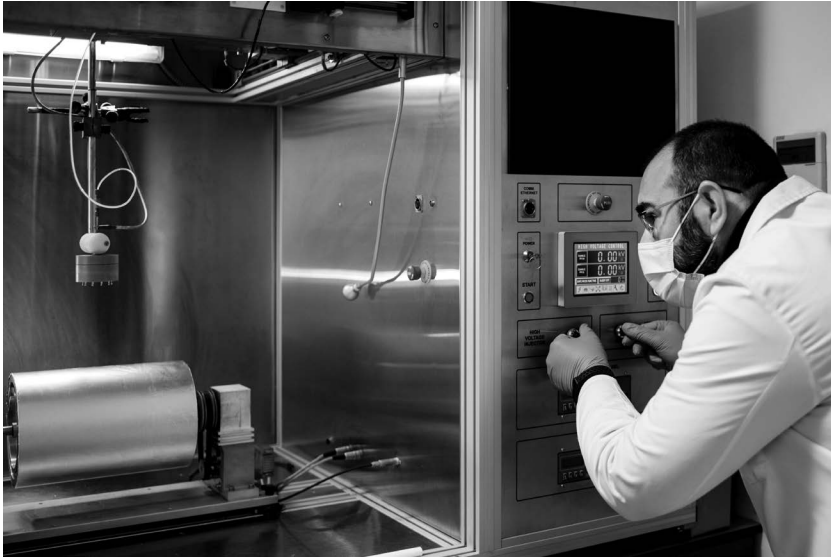
Figure 1.1 A lab technician tests nanofibers on an electrospinning machine.
