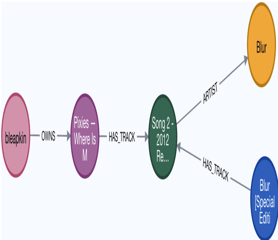
Figure 1-15. Cypher query result showing all the graph data after using the MERGE clause
