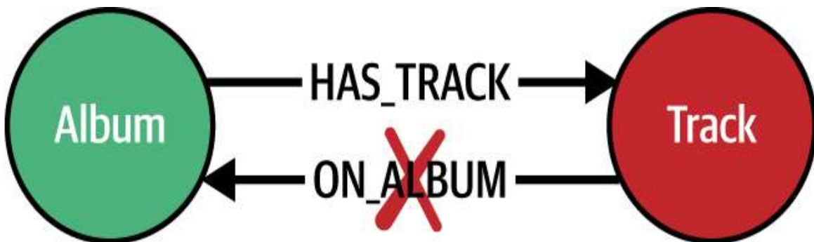
Figure 3-24. Do not add redundant relationships to navigate in the opposite direction.
