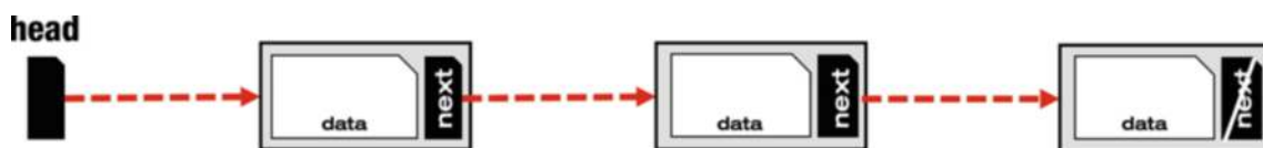
Figure 4.6: A simple view of a singly-linked list. The head points to the first node, and each node points to the next node in the sequence
