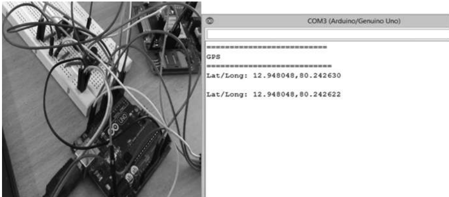
FIGURE 2.5 Collecting the location information through GPS Module on COM3 port.
