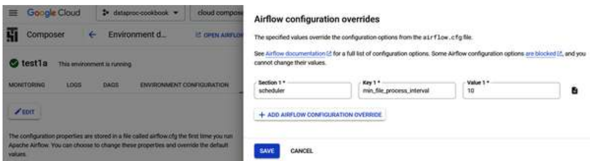
Figure 12-18. Configuring the minimum file process interval in overrides
