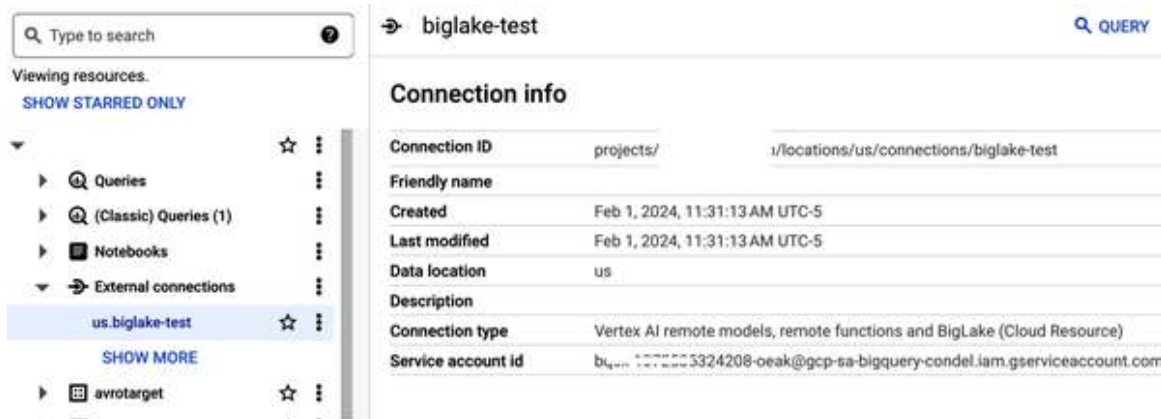
Figure 7-7. Connection ID and service account ID under connection info
