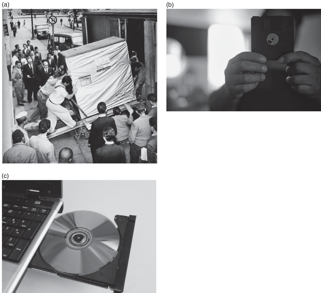
Figure 1.2 Photos of various types of older data storage. (a) The shipping of IBM's first hard drive, holding 5 MB and taking up the size of two refrigerators. (b) A 3.5-inch floppy disk, the main external data storage format in the 1980s and 1990s. (c) A CD-ROM inserted into a laptop's CD drive. These were commonly used in the 1990s and 2000s for data storage and were the main medium for holding music albums.
