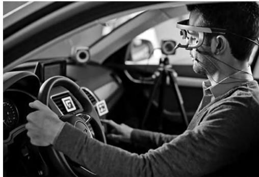
**FIGURE 9.9** Driver's eye-tracking devices [17].
