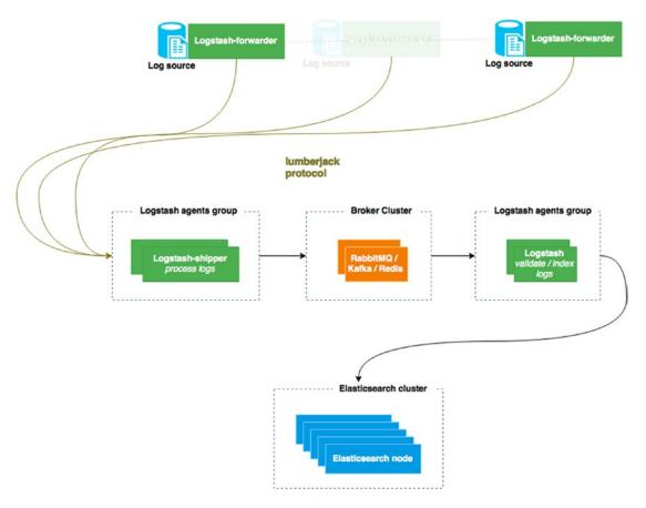
Figure 4-3. Logstash logging platform typical architecture
