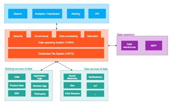
Figure 3-1. Hadoop-based data architecture
