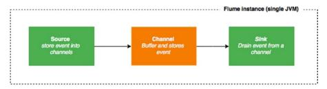
Figure 4-2. Flume architecture
