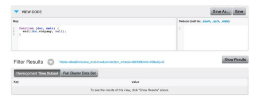
Figure 2-12. Couchbase console view implementation
