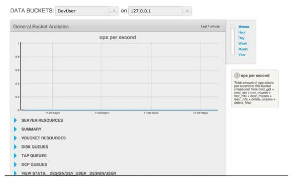
Figure 2-8. Couchbase bucket monitoring
