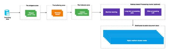
Figure 4-1. Anatomy of a typical data ingesting architecture
