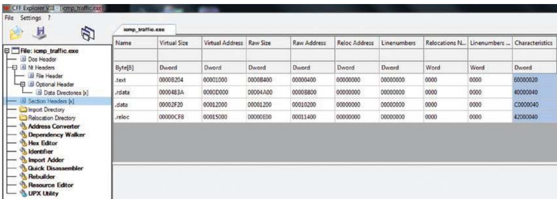
Figure 10-10. The Section Headers of a malware sample
