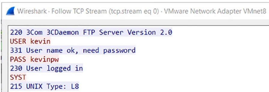
Figure 3-20. The TCP stream view in Wireshark
