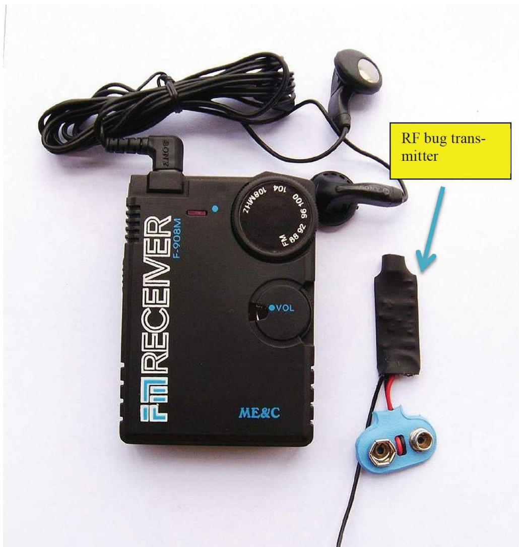
Wireless bug covert RF FM kit – Receiver, headphones, audio bug transmitter with 9v battery attachment
