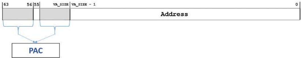
Figure 15.3: Layout of the virtual address with PAC
