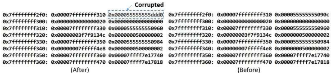
Figure 11.8: The memory dump for a corrupted stack with another pattern
