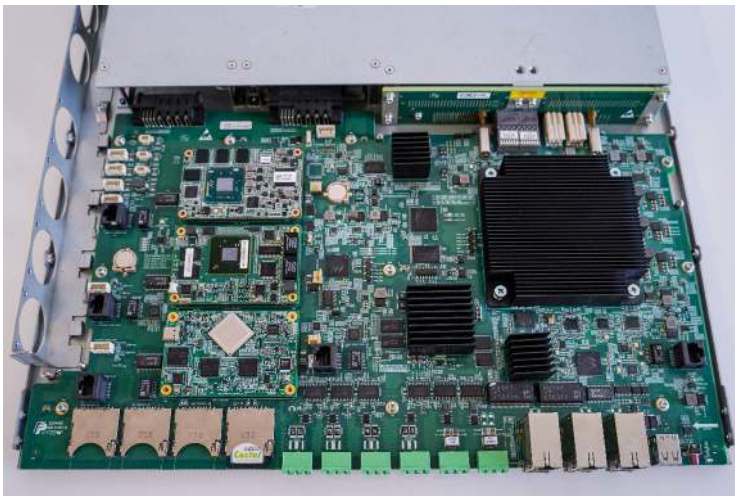
Fig. 7.51 Design view of an industrial Internet mimic edge gateway
